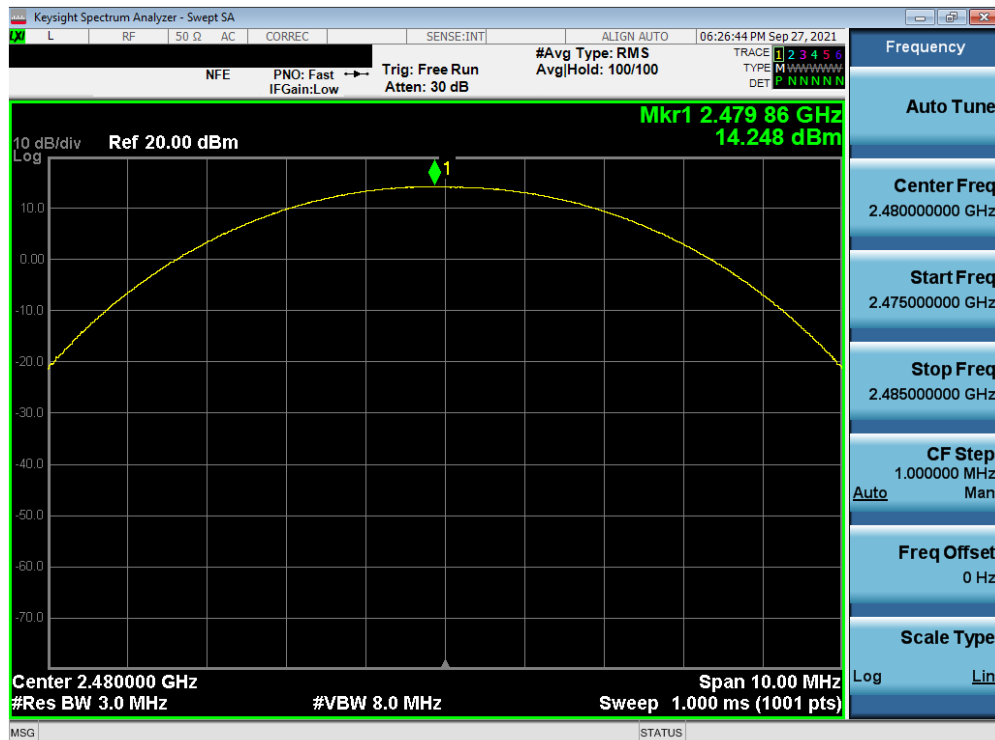
Plot 7-12. Peak Conducted Power (1Mbps – Ch. 78)
