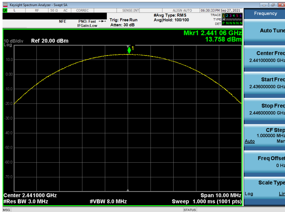
Plot 7-14. Peak Conducted Power (2Mbps – Ch. 39)
