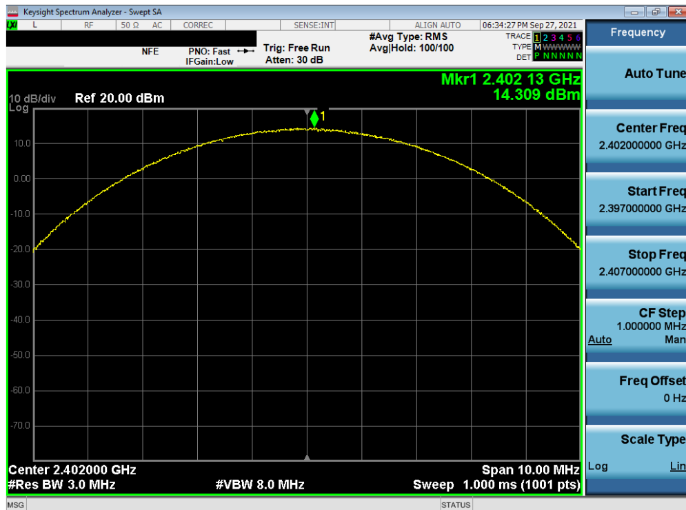
Plot 7-16. Peak Conducted Power (3Mbps – Ch. 0)
