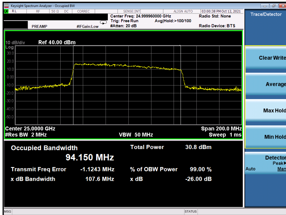
Plot 7-11. Ant 2 Occupied Bandwidth Plot (100MHz-1CC – 16QAM – Mid Channel)
