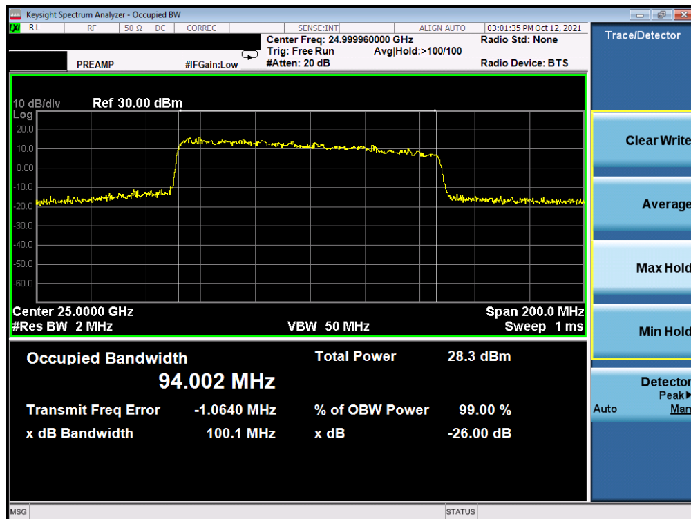
Plot 7-12. Ant 2 Occupied Bandwidth Plot (100MHz-1CC – 64QAM – Mid Channel)
