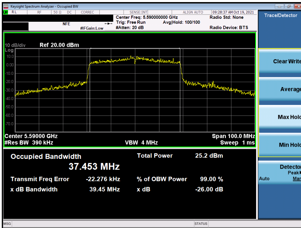
Plot 7-44. 26dB Bandwidth Plot SISO ANT1 (40MHz BW 802.11ax (UNII Band 2C) – Ch. 118)
