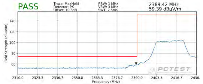
Plot 7-98. Radiated Restricted Lower Band Edge Measurement SISO ANT2 (Peak – 242 Tones)
