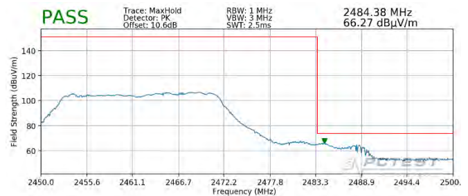
Plot 7-92. Radiated Restricted Upper Band Edge Measurement SISO ANT1 (Peak – 242 Tones)
