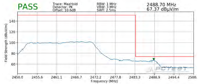
Plot 7-102. Radiated Restricted Upper Band Edge Measurement SISO ANT2 (Peak – 242 Tones)
