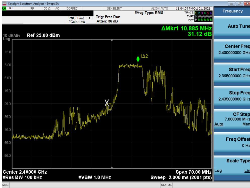
Plot 7-30. Band Edge Plot SISO ANT2 (802.11ax OFDMA – 106 Tones – Ch. 1)
