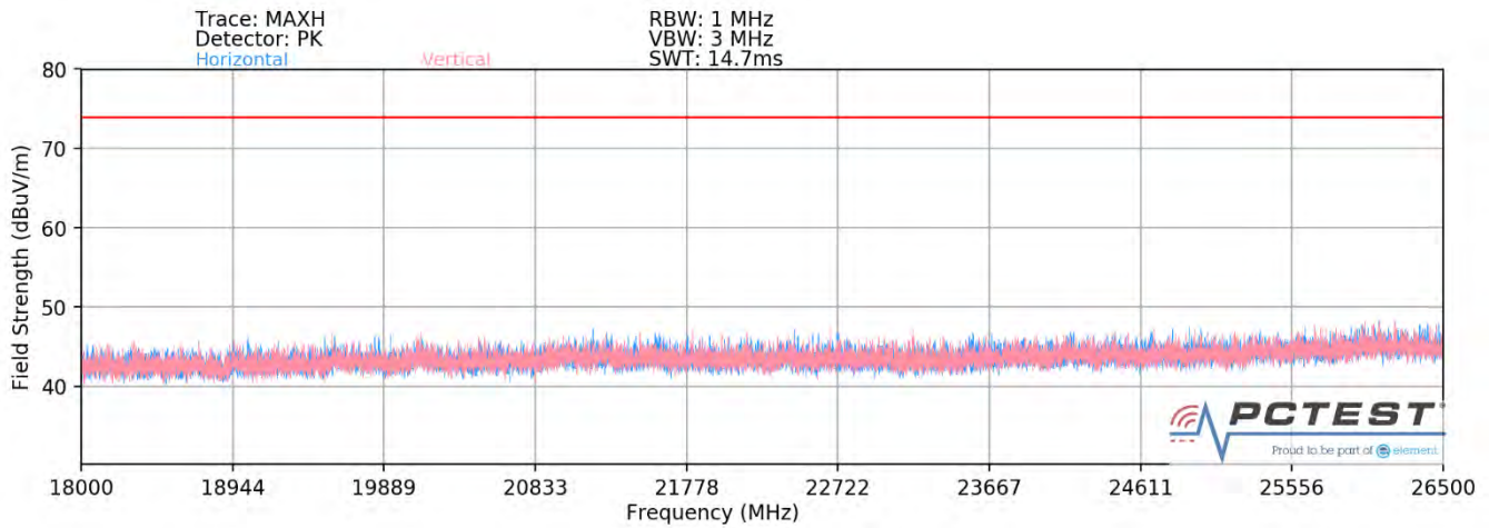
Plot 7-81. Radiated Spurious Plot above 18GHz MIMO (802.11ax OFDMA – 106 Tones)
