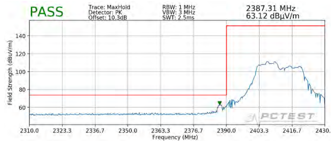
Plot 7-84. Radiated Restricted Lower Band Edge Measurement SISO ANT1 (Peak – 106 Tones)
