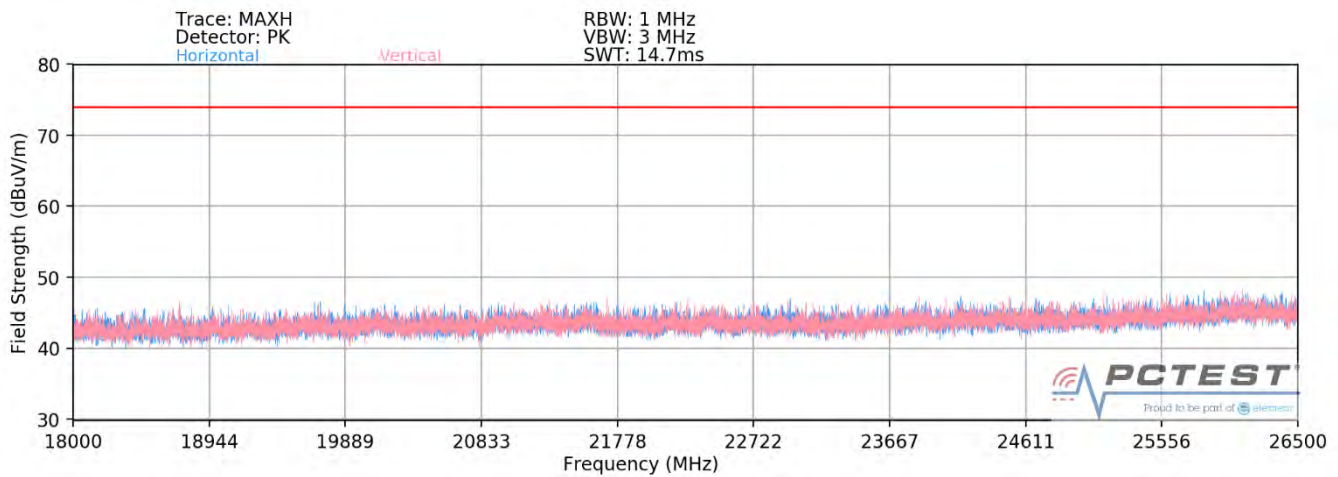
Plot 7-66. Radiated Spurious Plot above 18GHz SISO ANT1 (802.11ax OFDMA – 242 Tones)
