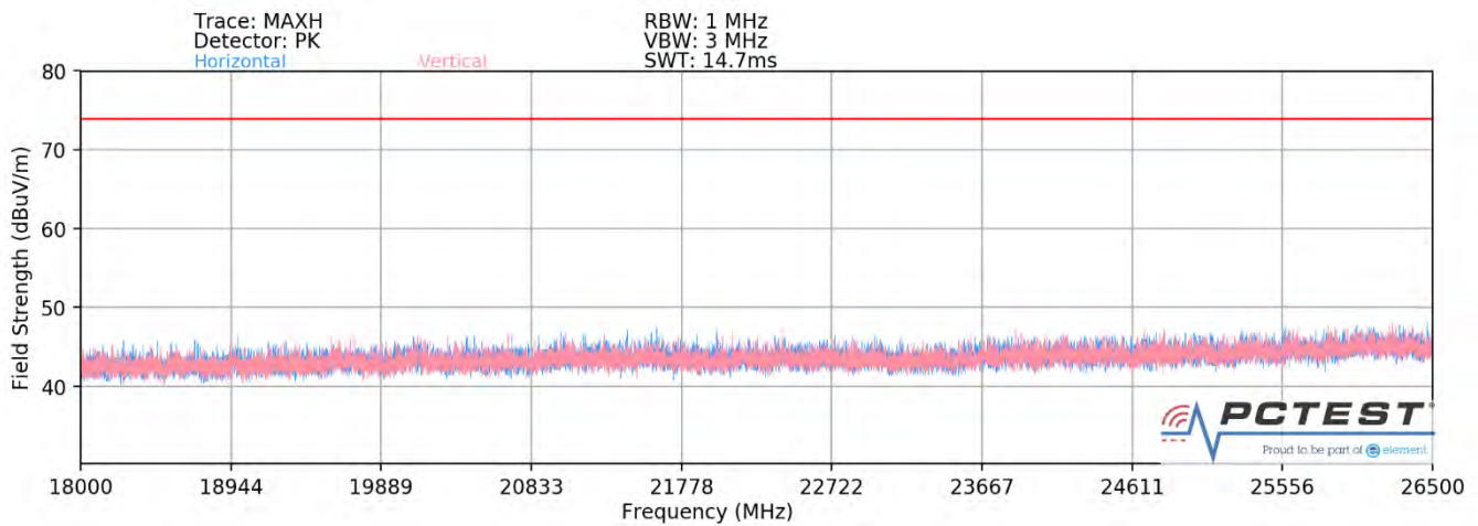
Plot 7-82. Radiated Spurious Plot above 18GHz MIMO (802.11ax OFDMA – 242 Tones)
