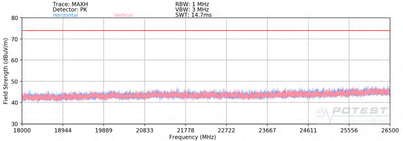
Plot 7-108. Radiated Spurious Plot above 18GHz SISO ANT1
