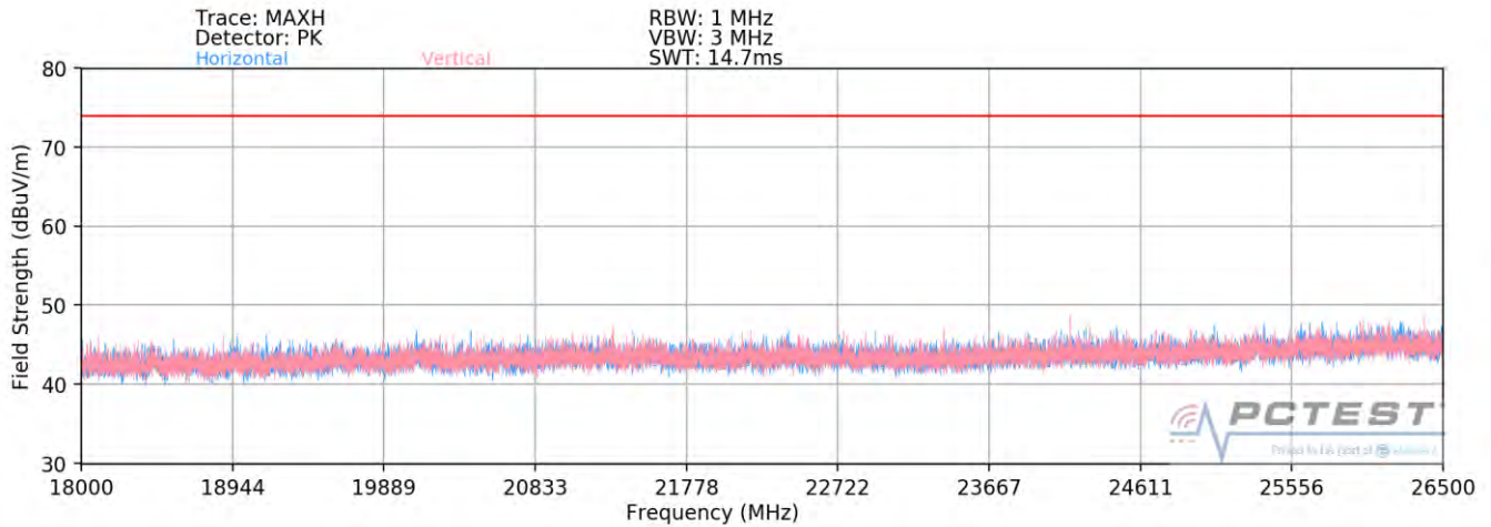
Plot 7-116. Radiated Spurious Plot above 18GHz MIMO/CDD
