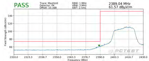
Plot 7-118. Radiated Restricted Lower Band Edge Measurement SISO ANT1 (Peak)
