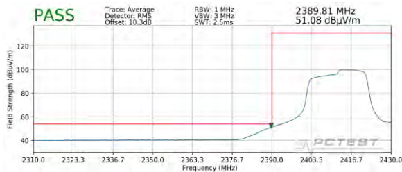
Plot 7-129. Radiated Restricted Lower Band Edge Measurement MIMO (Average)
