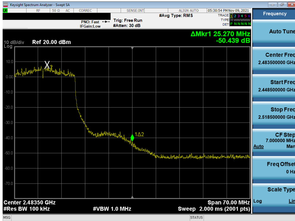
Plot 7-81. Band Edge Plot SISO ANT1 (802.11ax (2.4GHz) – Ch. 10)
