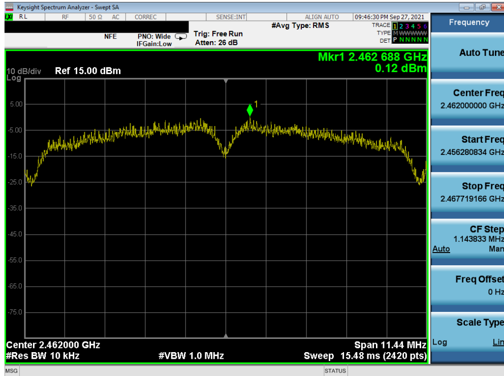
Plot 7-63. Power Spectral Density Plot MIMO ANT2 (802.11b) (2.4GHz) – Ch. 11)
