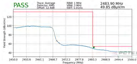
Plot 7-119. Radiated Restricted Lower Band Edge Measurement SISO ANT1 (Average)
