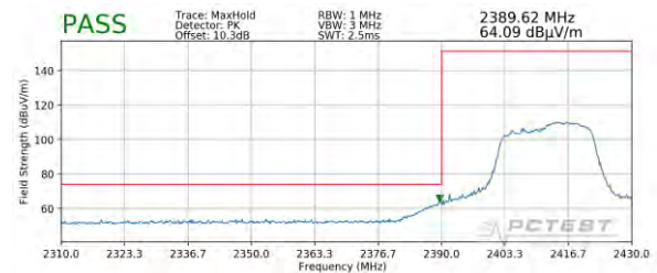
Plot 7-130. Radiated Restricted Lower Band Edge Measurement MIMO (Peak)
