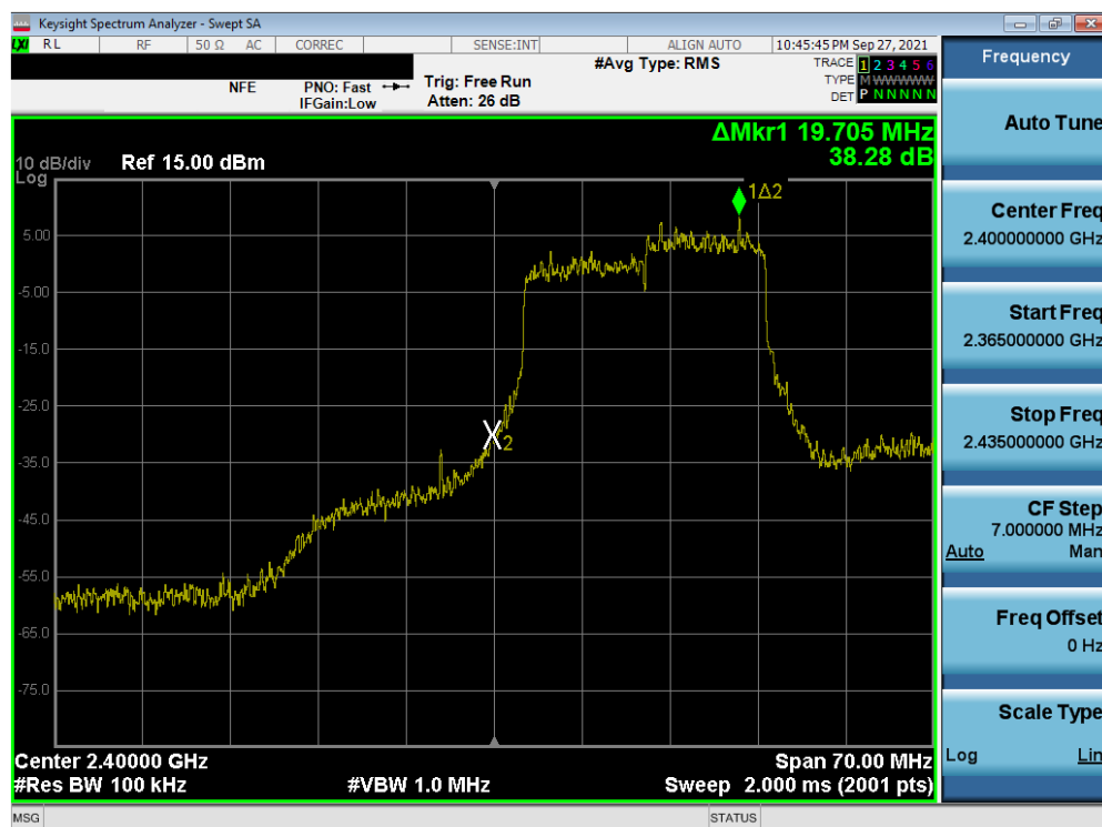
Plot 7-80. Band Edge Plot SISO ANT1 (802.11ax (2.4GHz) – Ch. 1)
