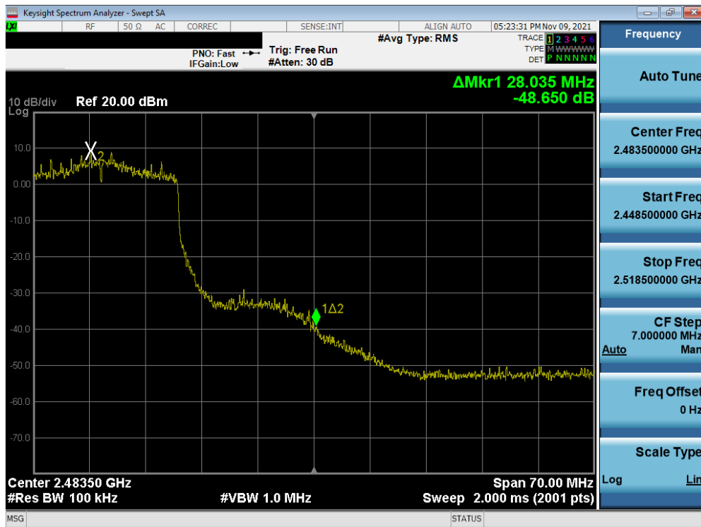
Plot 7-91. Band Edge Plot SISO ANT2 (802.11ax (2.4GHz) – Ch. 10)
