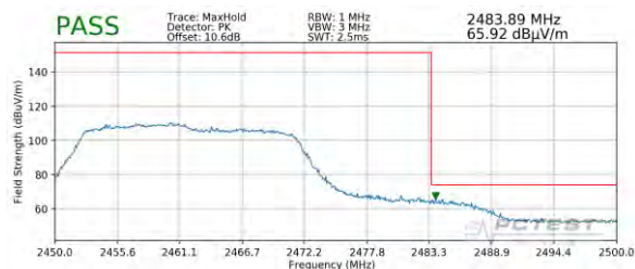
Plot 7-134. Radiated Restricted Lower Band Edge Measurement MIMO (Peak)
