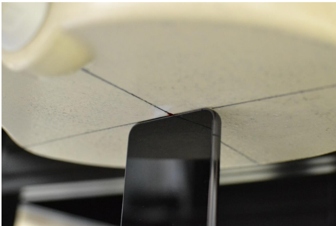
Test Setup Photo 15 – Body, Bottom Edge at 0 mm
