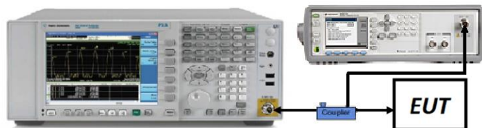
Figure 7-3. Test Instrument & Measurement Setup
