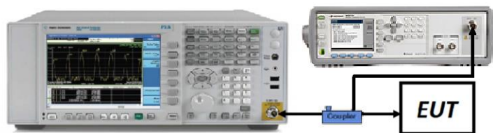
Figure 7-5. Test Instrument & Measurement Setup
