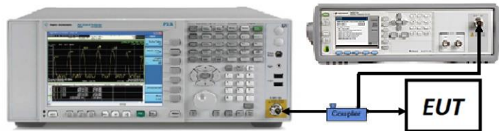
Figure 7-2. Test Instrument & Measurement Setup
