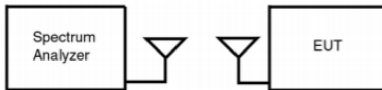
Figure 7-1. Test Instrument and Measurement Setup
