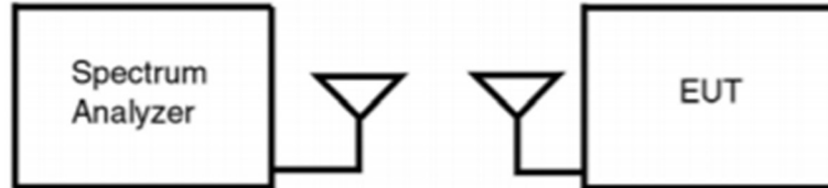
Figure 7-2. Test Instrument and Measurement Setup
