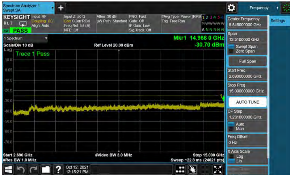
Plot 7-13. Conducted Spurious Plot (LTE Band 41(PC2) - 20MHz QPSK - RB Size 1, RB Offset 0 - Mid Channel)
