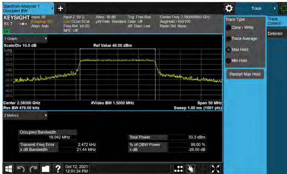
Plot 7-2. Occupied Bandwidth Plot (LTE Band 41(PC2) - 20MHz 16-QAM - Full RB)
