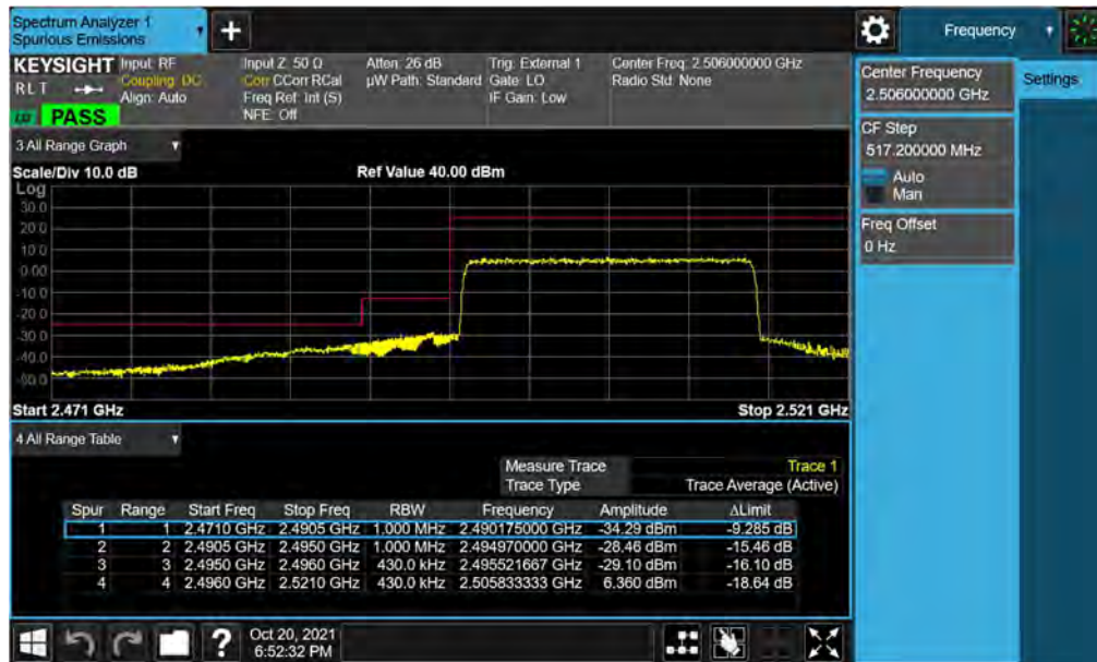
Plot 7-18. Lower ACP Plot (LTE Band 41(PC2) - 20MHz QPSK – Full RB)
