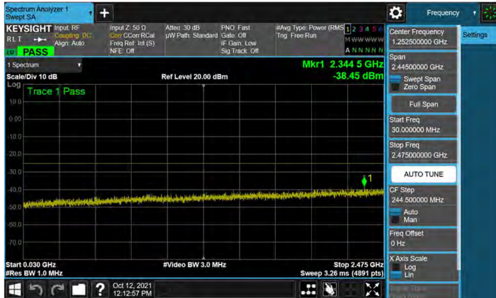
Plot 7-9. Conducted Spurious Plot (LTE Band 41(PC2) - 20MHz QPSK - RB Size 1, RB Offset 0 - Low Channel)
