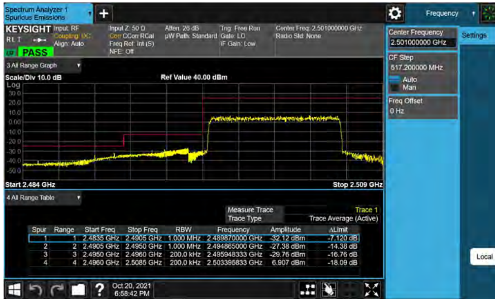
Plot 7-22. Lower ACP Plot (LTE Band 41(PC2) - 10MHz QPSK - Full RB)
