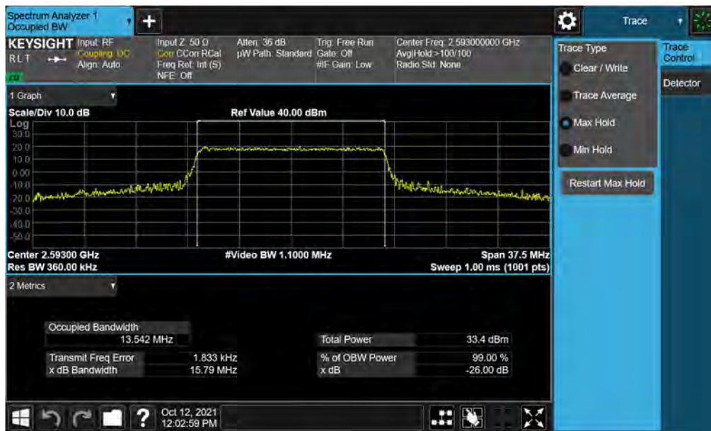
Plot 7-4. Occupied Bandwidth Plot (LTE Band 41(PC2) - 15MHz 16-QAM - Full RB)
