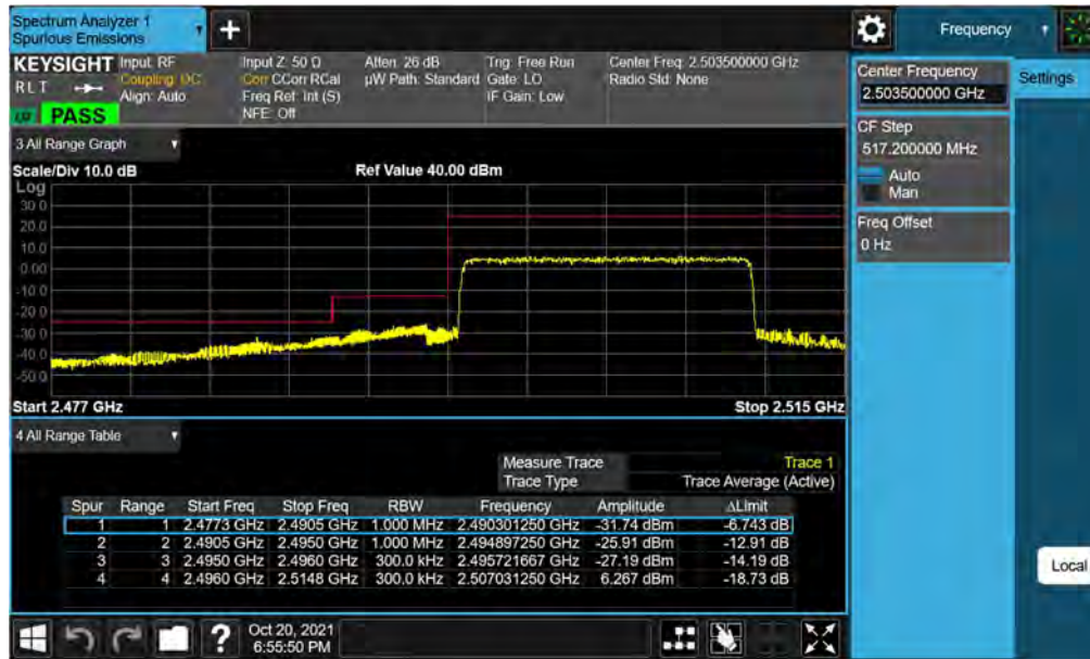
Plot 7-20. Lower ACP Plot (LTE Band 41(PC2) - 15MHz QPSK - Full RB)
