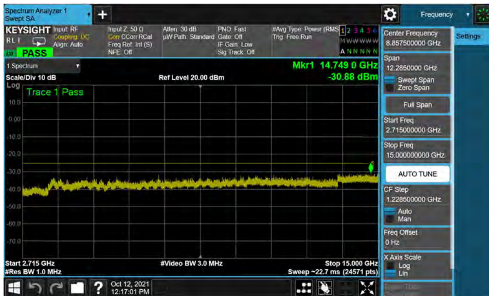
Plot 7-16. Conducted Spurious Plot (LTE Band 41(PC2) - 20MHz QPSK - RB Size 1, RB Offset 0 - High Channel)
