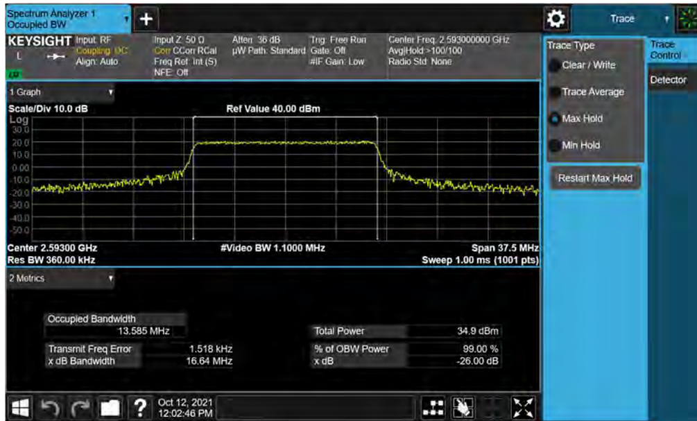
Plot 7-3. Occupied Bandwidth Plot (LTE Band 41(PC2) - 15MHz QPSK - Full RB)
