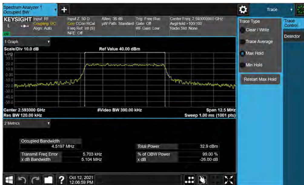
Plot 7-8. Occupied Bandwidth Plot (LTE Band 41(PC2) - 5MHz 16-QAM - Full RB)
