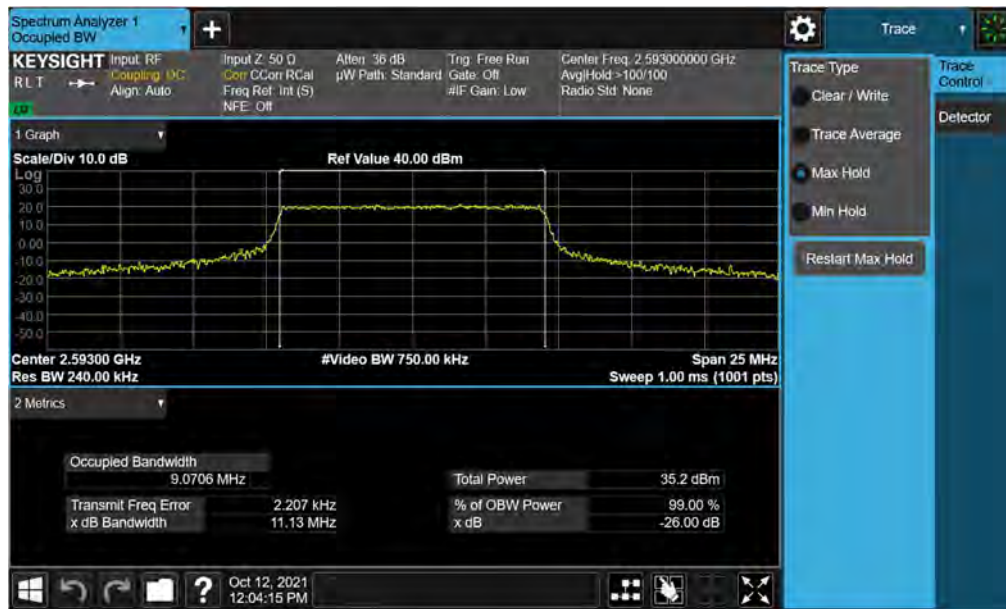
Plot 7-5. Occupied Bandwidth Plot (LTE Band 41(PC2) - 10MHz QPSK - Full RB)
