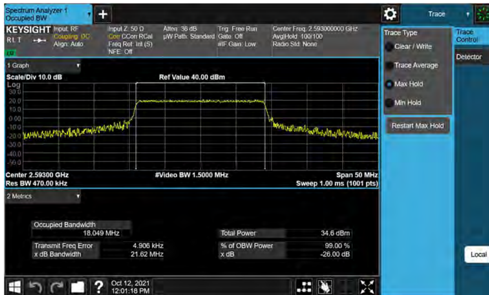
Plot 7-1. Occupied Bandwidth Plot (LTE Band 41(PC2) - 20MHz QPSK - Full RB)
