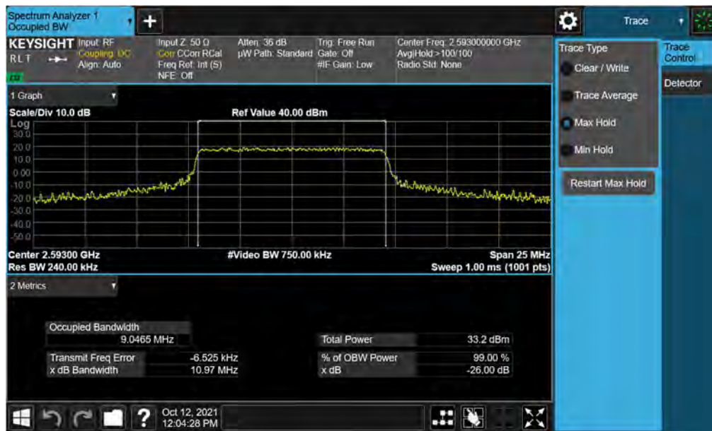
Plot 7-6. Occupied Bandwidth Plot (LTE Band 41(PC2) - 10MHz 16-QAM - Full RB)
