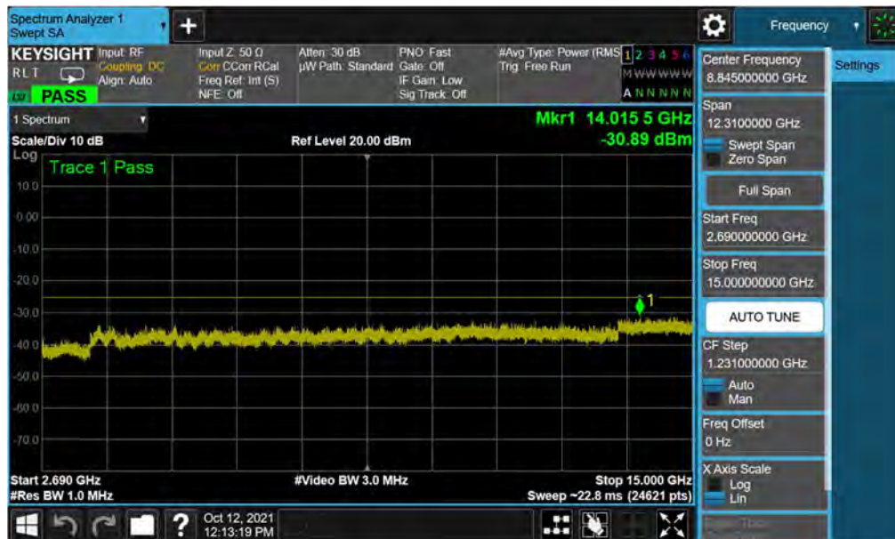
Plot 7-10. Conducted Spurious Plot (LTE Band 41(PC2) - 20MHz QPSK - RB Size 1, RB Offset 0 - Low Channel)
