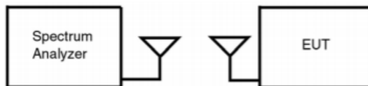
Figure 7-1. Test Instrument and Measurement Setup
