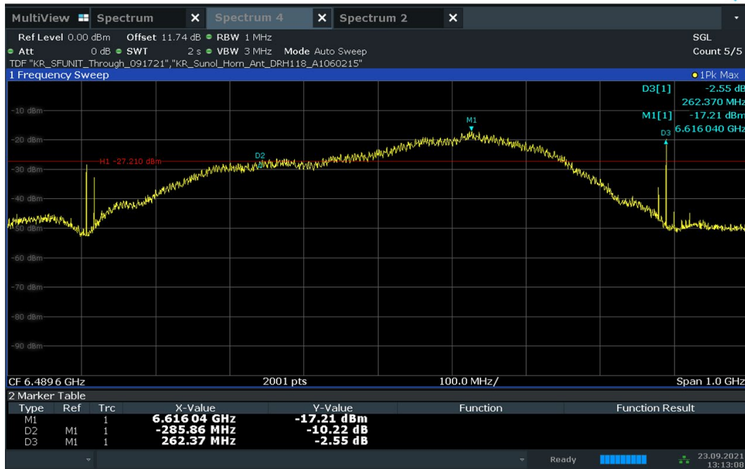
Plot 7-39. 10dBc Bandwidth – CH.5 – SP3 – Preamble 11
