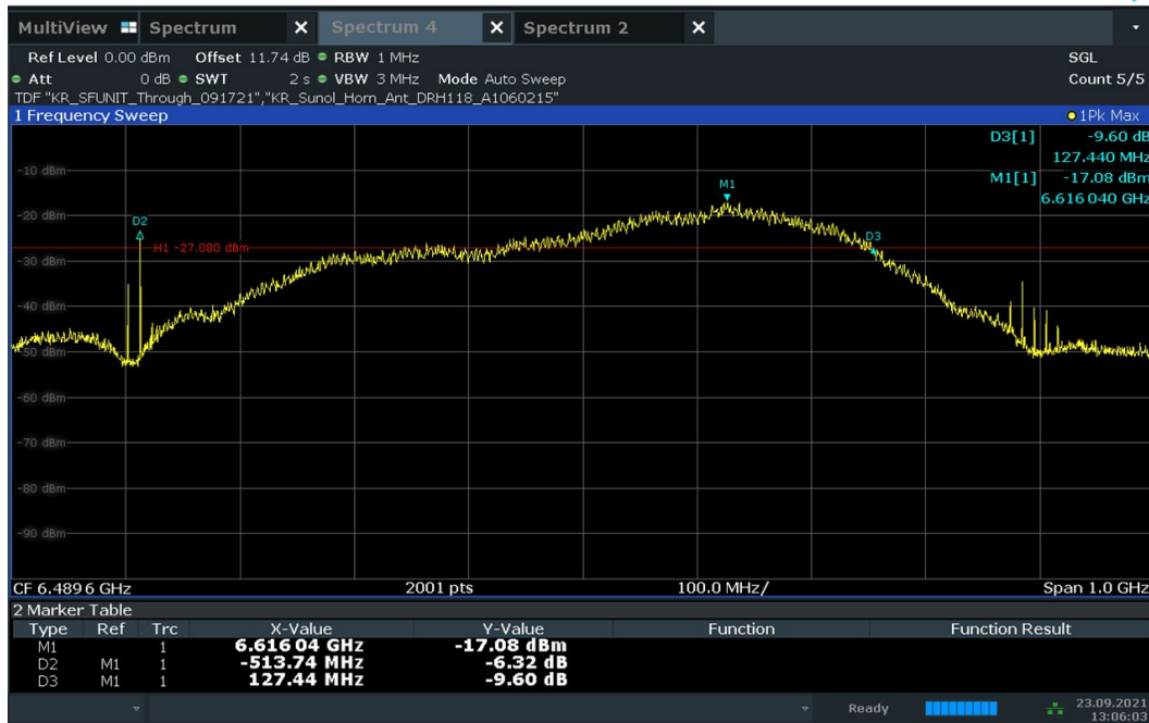
Plot 7-33. 10dBc Bandwidth – CH.5 – SP3 – Preamble 9
