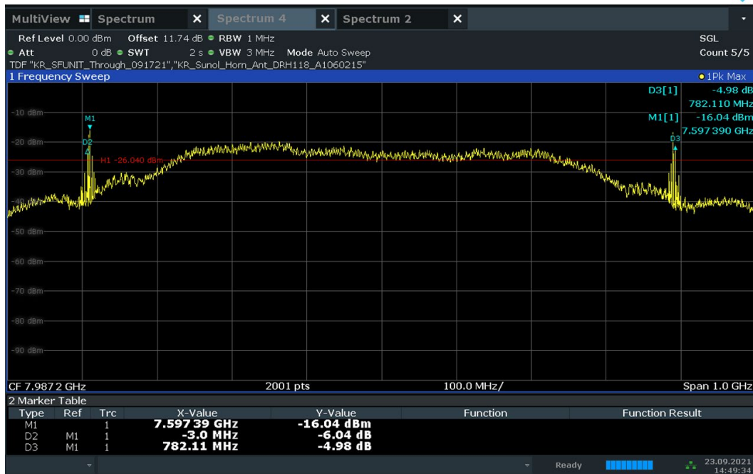
Plot 7-26. 10dBc Bandwidth – CH.9 – SP1 – Preamble 12
