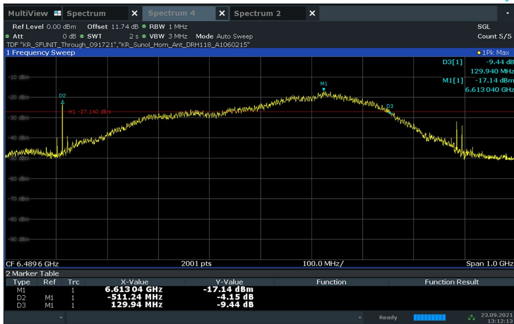
Plot 7-38. 10dBc Bandwidth – CH.5 – SP1 – Preamble 11
