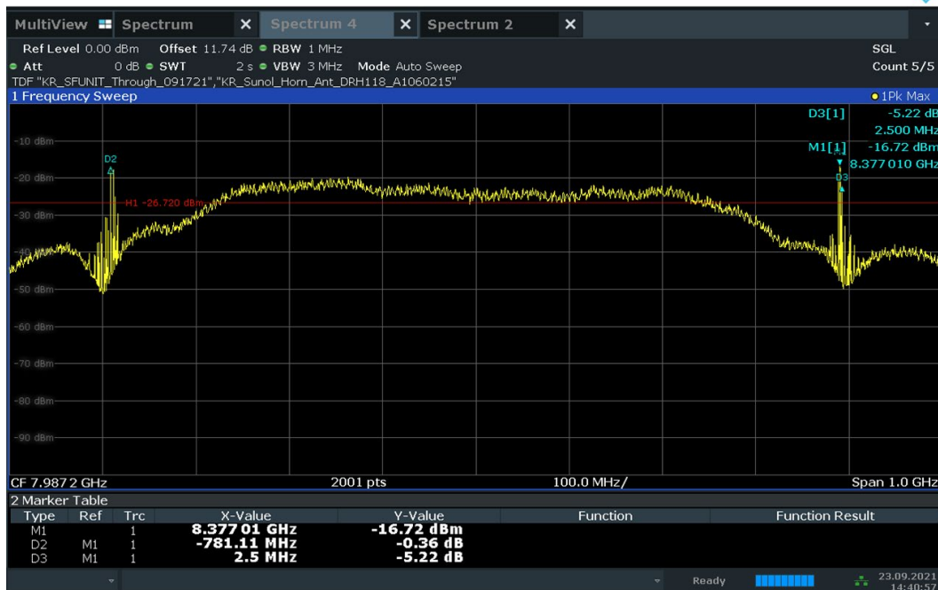
Plot 7-18. 10dBc Bandwidth – CH.9 – SP3 – Preamble 9
