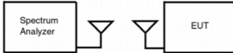
Figure 7-2. Test Instrument and Measurement Setup
