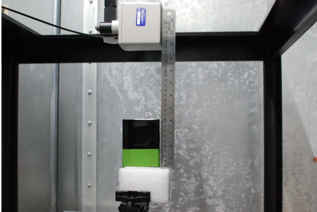
Test Setup Photo 27 E-field, Top edge, 15cm
