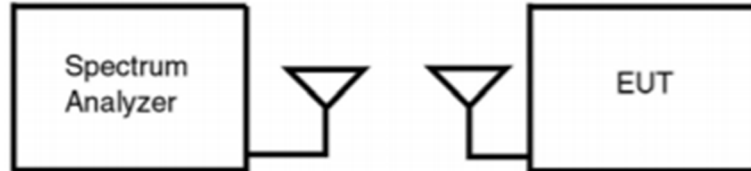
Figure 7-2. Test Instrument and Measurement Setup
