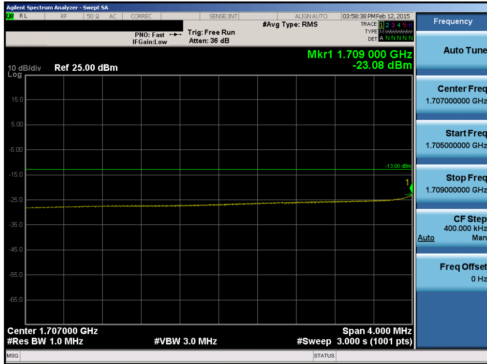
Plot 6-56. Lower Extended Band Edge Plot (Band 4 – 10.0MHz QPSK – RB Size 50)
