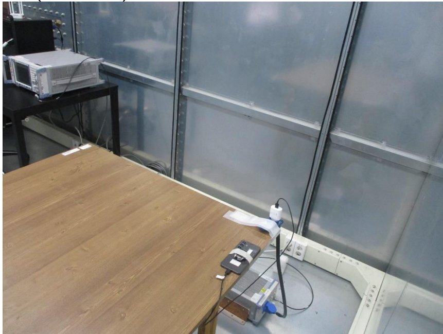
AC LINE CONDUCTED REAR TEST PHOTO WPT(Test Case 5)
