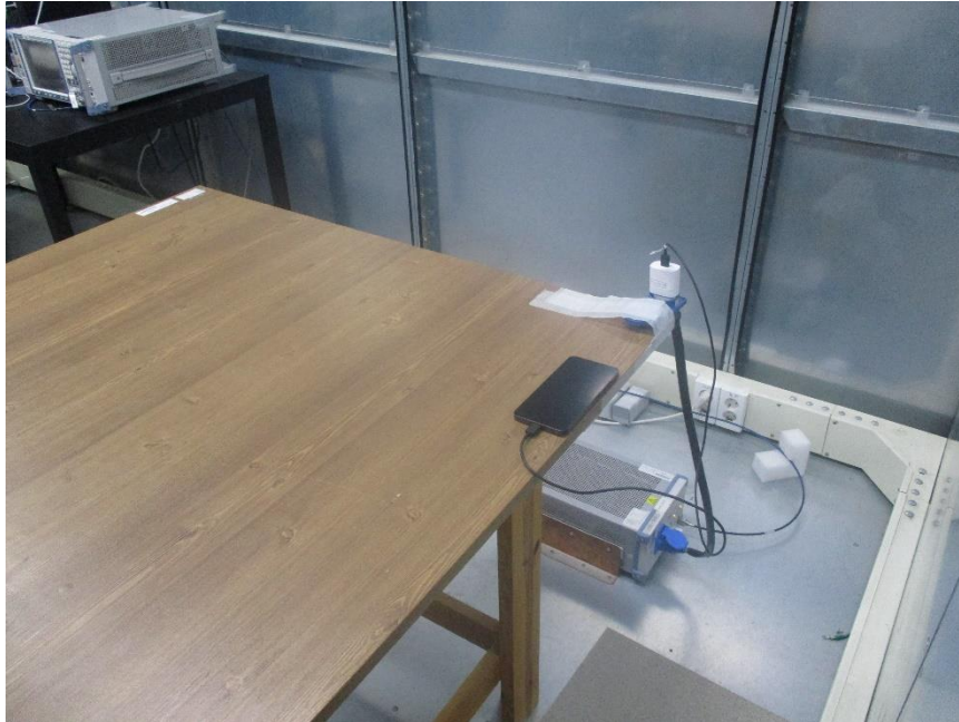
AC LINE CONDUCTED REAR TEST PHOTO
