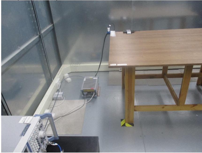
AC LINE CONDUCTED FRONT TEST PHOTO WPT(Test Case 4)
