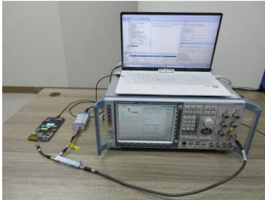
Test setup photo-1 (7-1(a) WLAN 2.4GHz Time-varying Tx Power Transmission, Change in Call, Change in DSI)
