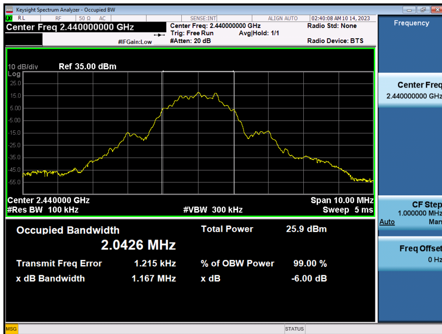
6 dB Bandwidth plot (Mid-CH 19)
