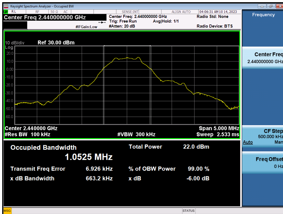
6 dB Bandwidth plot (Mid-CH 19)
