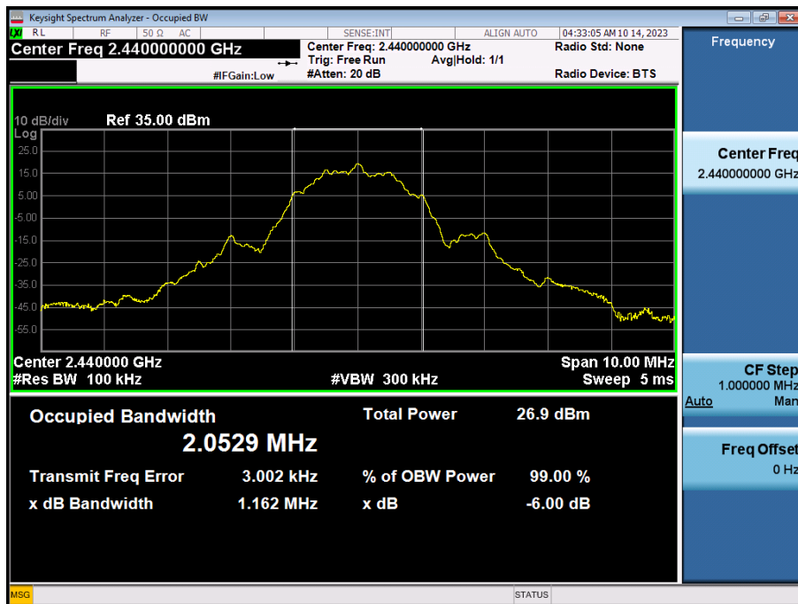
6 dB Bandwidth plot (Mid-CH 19)
