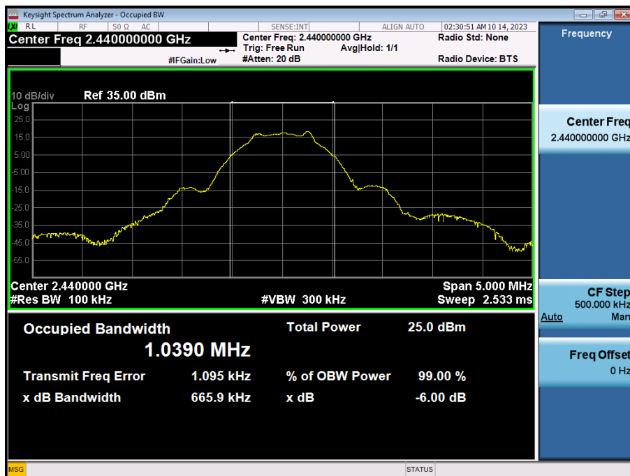
6 dB Bandwidth plot (Mid-CH 19)
