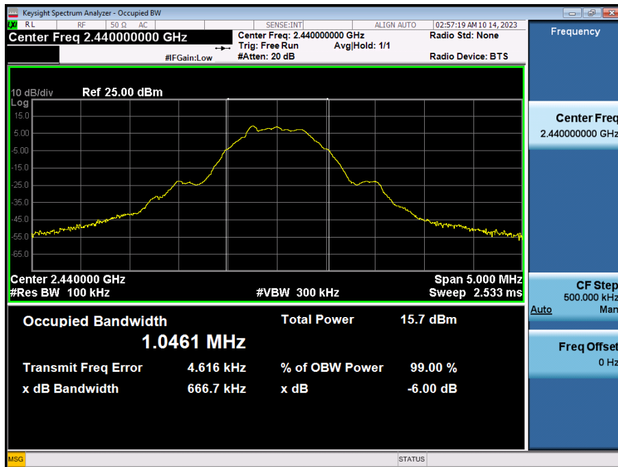
6 dB Bandwidth plot (Mid-CH 19)
