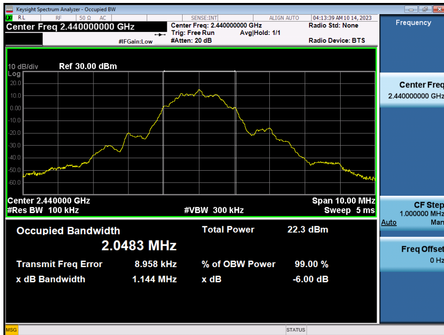
6 dB Bandwidth plot (Mid-CH 19)
