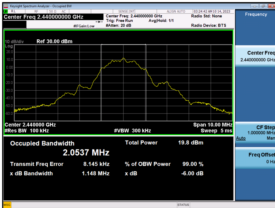
6 dB Bandwidth plot (Mid-CH 19)
