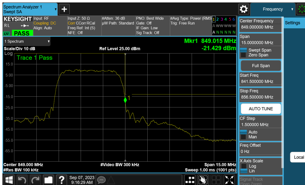
Plot 7-90. Upper Band Edge Plot (WCDMA Cell – Ch. 4233 – Ant 6)
