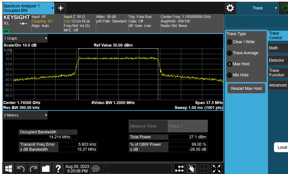
Plot 7-85. Occupied Bandwidth Plot (NR Band n66 - 15.0MHz CP-OFDM 16QAM - Full RB – Ant 7)
