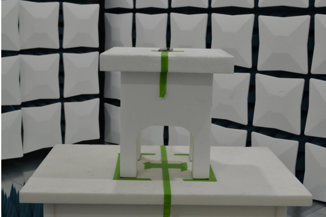
Figure 7. Test Setup – X Position – 1GHz-40GHz
