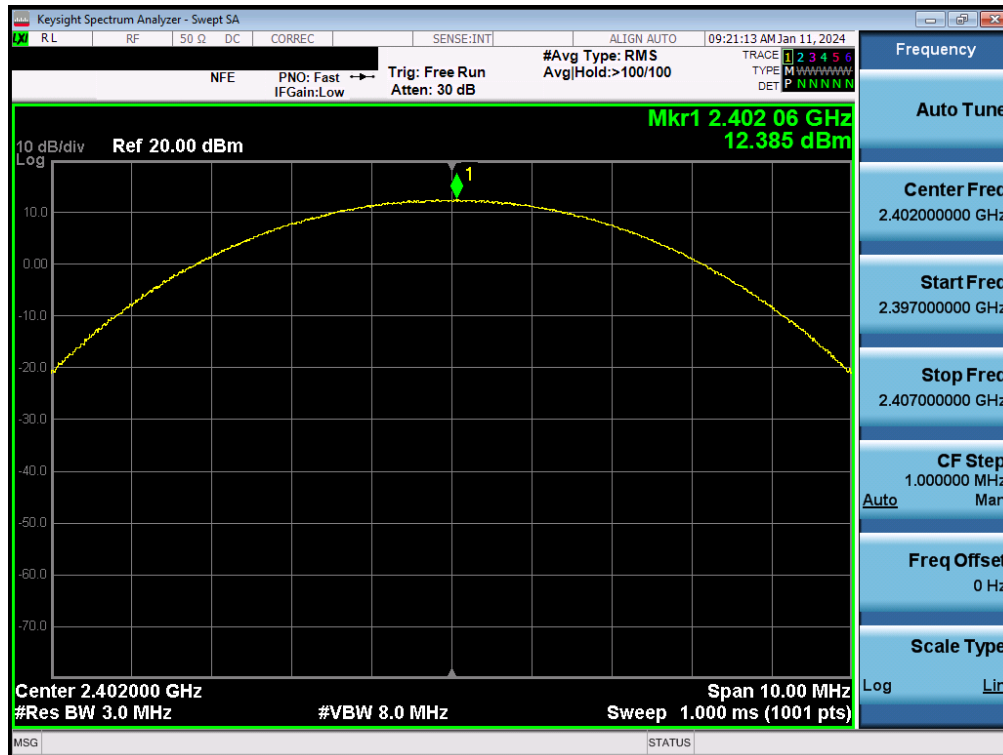
Plot 7-76. Peak Conducted Power (2Mbps – Ch. 0) – ANT1
