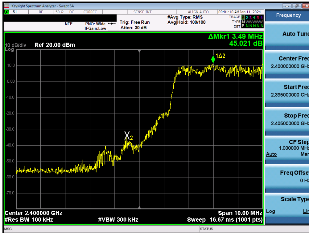
Plot 7-115. Band Edge Plot (Bluetooth with Hopping Enabled, 3 Mbps – Ch. 0) – ANT2
