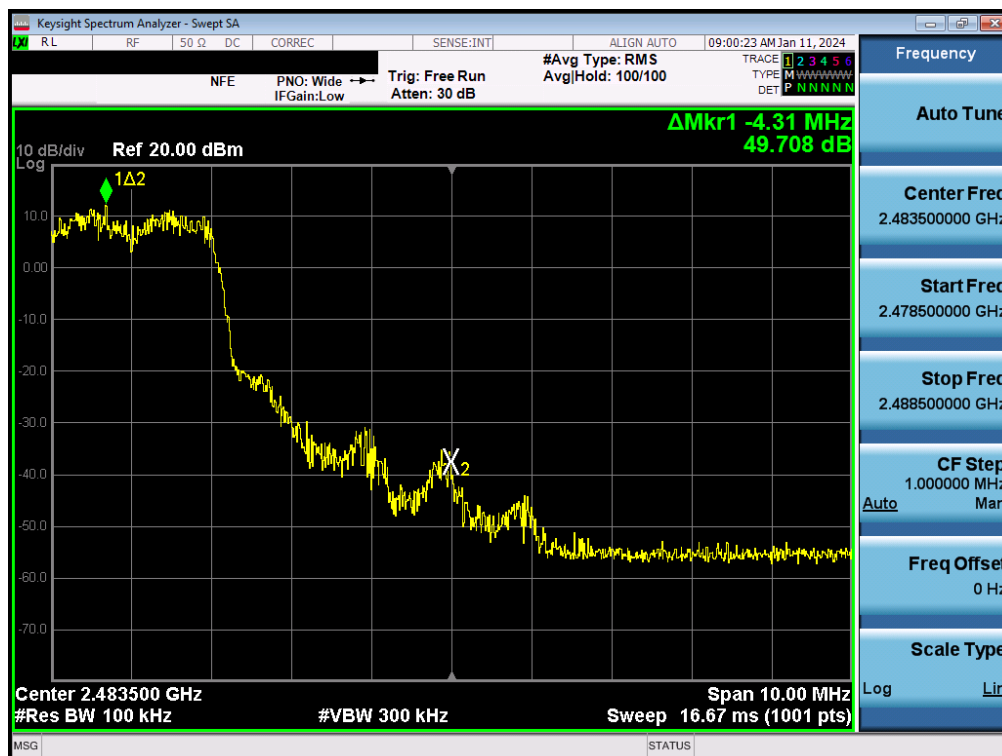
Plot 7-116. Band Edge Plot (Bluetooth with Hopping Enabled, 3 Mbps – Ch. 78) – ANT2
