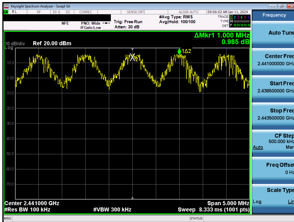
Plot 7-126. Channel Spacing Plot (Bluetooth) – ANT2
