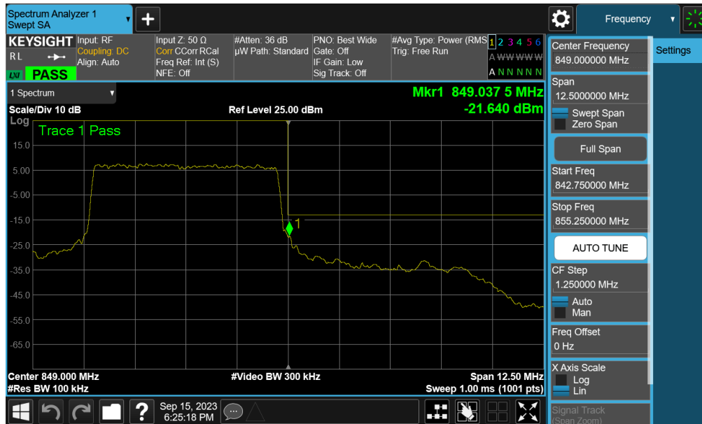
Plot 7-82. Upper Band Edge Plot (NR Band n26/5 – 5.0MHz QPSK - Full RB – Ant A)
