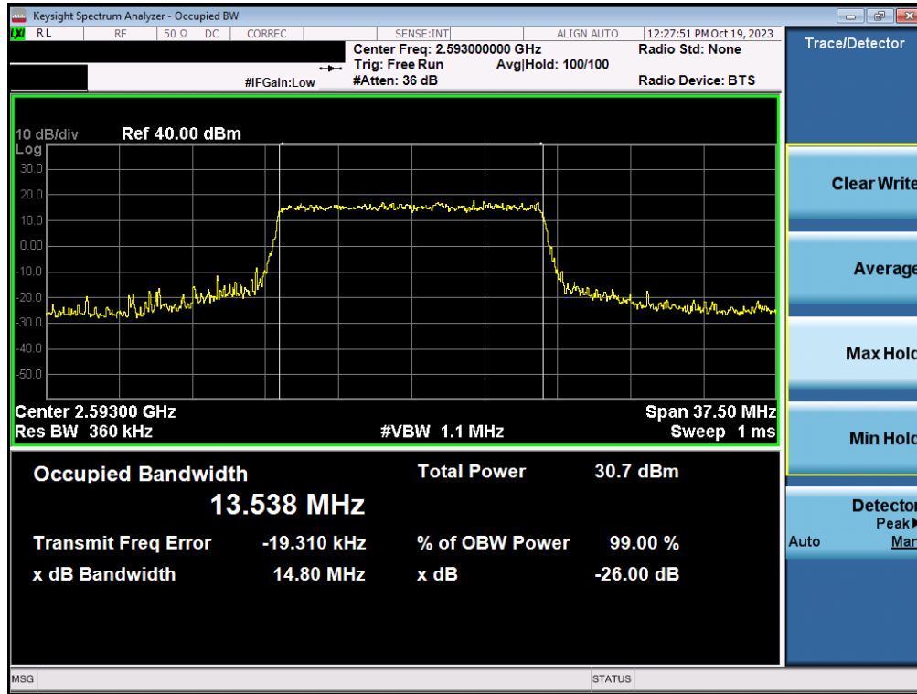
Plot 7-15. Occupied Bandwidth Plot (LTE Band 41(PC2) - 15MHz QPSK - Full RB - Ant1)
