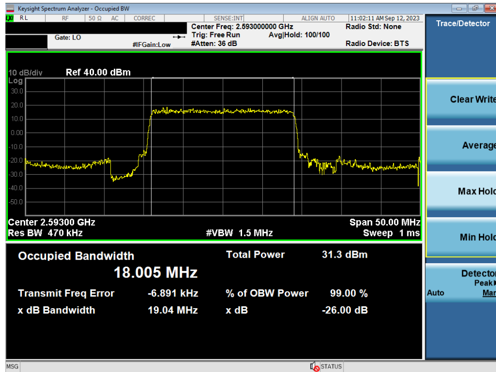
Plot 7-13. Occupied Bandwidth Plot (LTE Band 41(PC2) - 20MHz QPSK - Full RB - Ant1)
