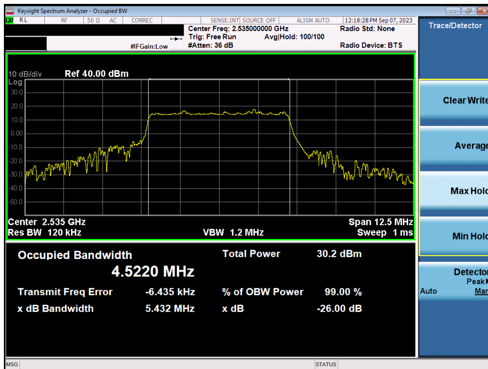
Plot 7-56. Occupied Bandwidth Plot (NR Band n7 - 5MHz \pi/2 BPSK - Full RB - Ant1)
