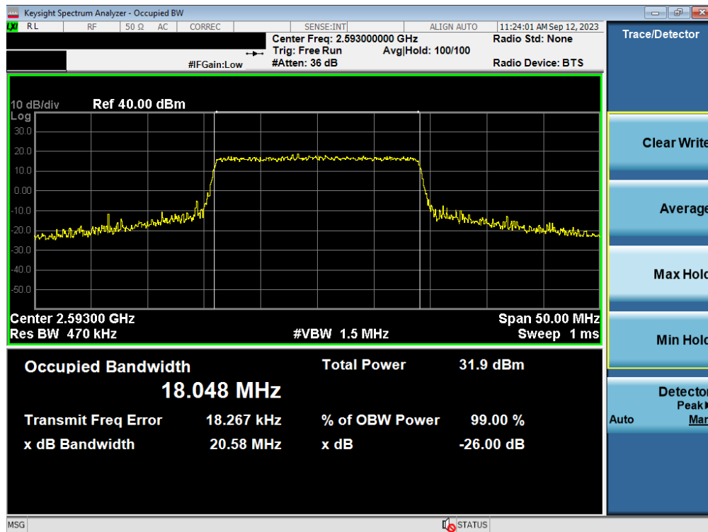
Plot 7-22. Occupied Bandwidth Plot (LTE Band 41(PC3)/38 - 20MHz 16-QAM - Full RB - Ant1)
