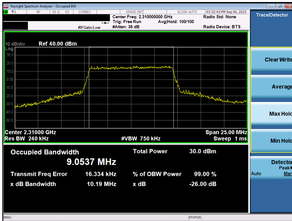
Plot 7-132. Occupied Bandwidth Plot (LTE Band 30 - 10MHz 16-QAM - Full RB - Ant2)
