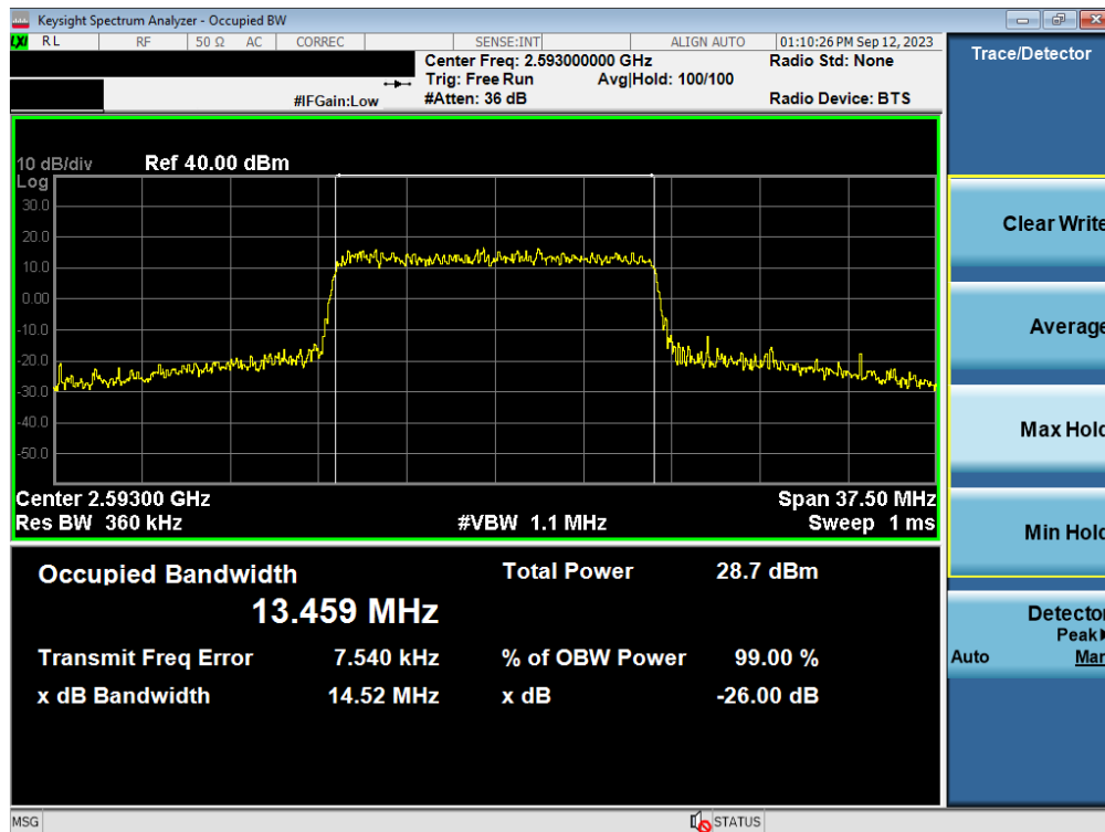
Plot 7-154. Occupied Bandwidth Plot (LTE Band 41(PC3)/38 - 15MHz 16-QAM - Full RB - Ant2)
