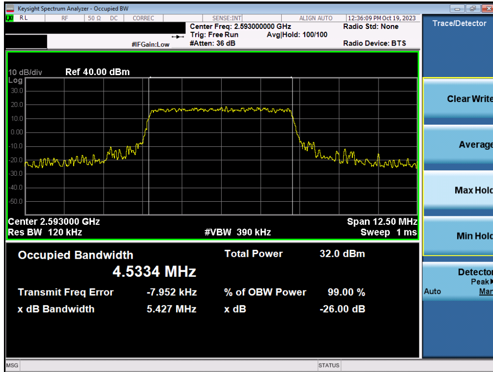
Plot 7-149. Occupied Bandwidth Plot (LTE Band 41(PC2) - 5MHz QPSK - Full RB - Ant2)
