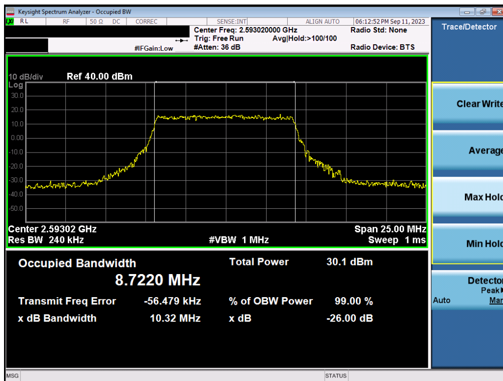
Plot 7-94. Occupied Bandwidth Plot (NR Band n41 - 10MHz 16-QAM - Full RB Configuration - Ant1)
