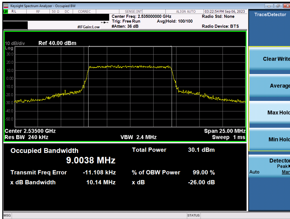
Plot 7-140. Occupied Bandwidth Plot (LTE Band 7 - 10MHz 16-QAM - Full RB - Ant2)
