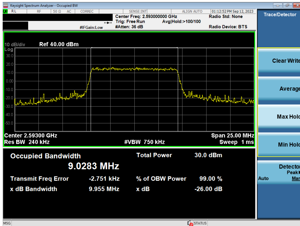
Plot 7-156. Occupied Bandwidth Plot (LTE Band 41(PC3)/38 - 10MHz 16-QAM - Full RB - Ant2)
