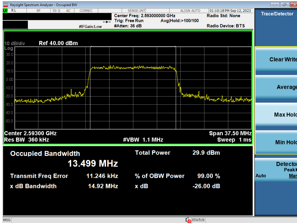
Plot 7-153. Occupied Bandwidth Plot (LTE Band 41(PC3)/38 - 15MHz QPSK - Full RB - Ant2)
