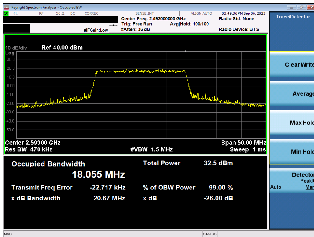
Plot 7-144. Occupied Bandwidth Plot (LTE Band 41(PC2) - 20MHz 16-QAM - Full RB - Ant2)
