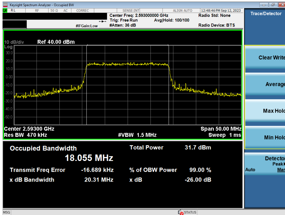
Plot 7-152. Occupied Bandwidth Plot (LTE Band 41(PC3)/38 - 20MHz 16-QAM - Full RB - Ant2)
