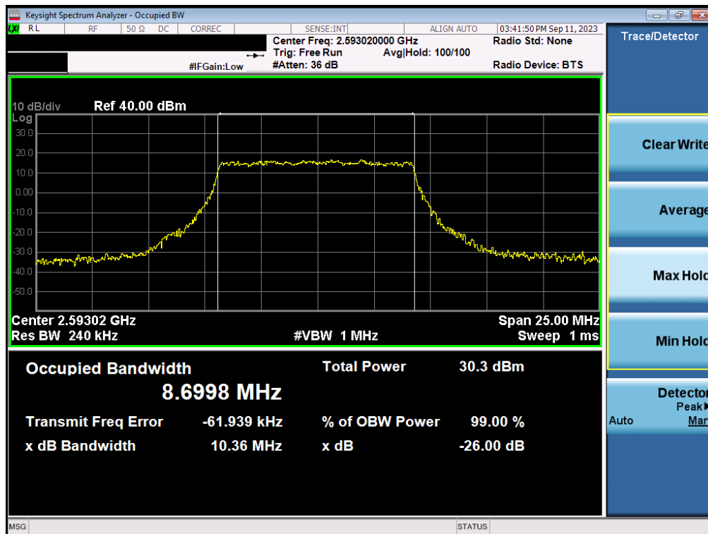
Plot 7-130. Occupied Bandwidth Plot (NR Band n41 Switching - 10MHz 16-QAM - Full RB Configuration - Ant1)
