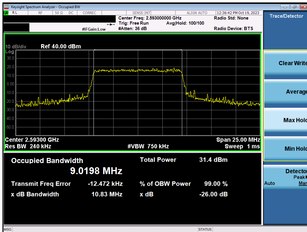
Plot 7-148. Occupied Bandwidth Plot (LTE Band 41(PC2) - 10MHz 16-QAM - Full RB - Ant2)
