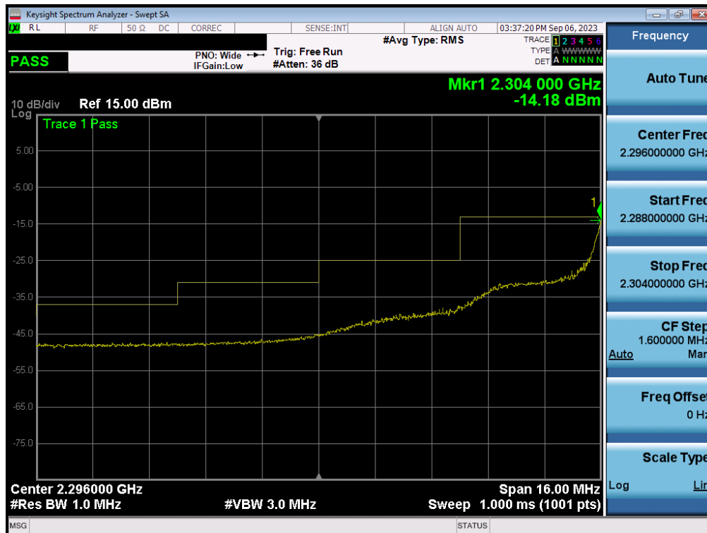
Plot 7-282. Extended Lower Band Edge Plot (LTE Band 30 - 5MHz QPSK – Full RB - Ant2)
