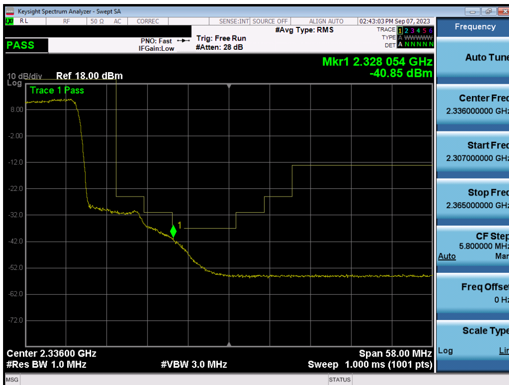
Plot 7-298. Extended Upper Band Edge Plot (NR Band n30 - 10MHz CP-OFDM-QPSK – Full RB - Ant2)
