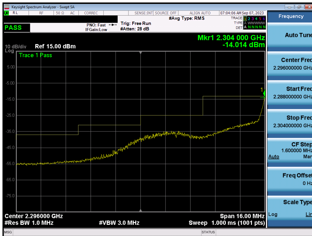
Plot 7-272. Extended Lower Band Edge Plot (NR Band n30 - 5MHz – DFT-s-QPSK – Full RB - Ant1)
