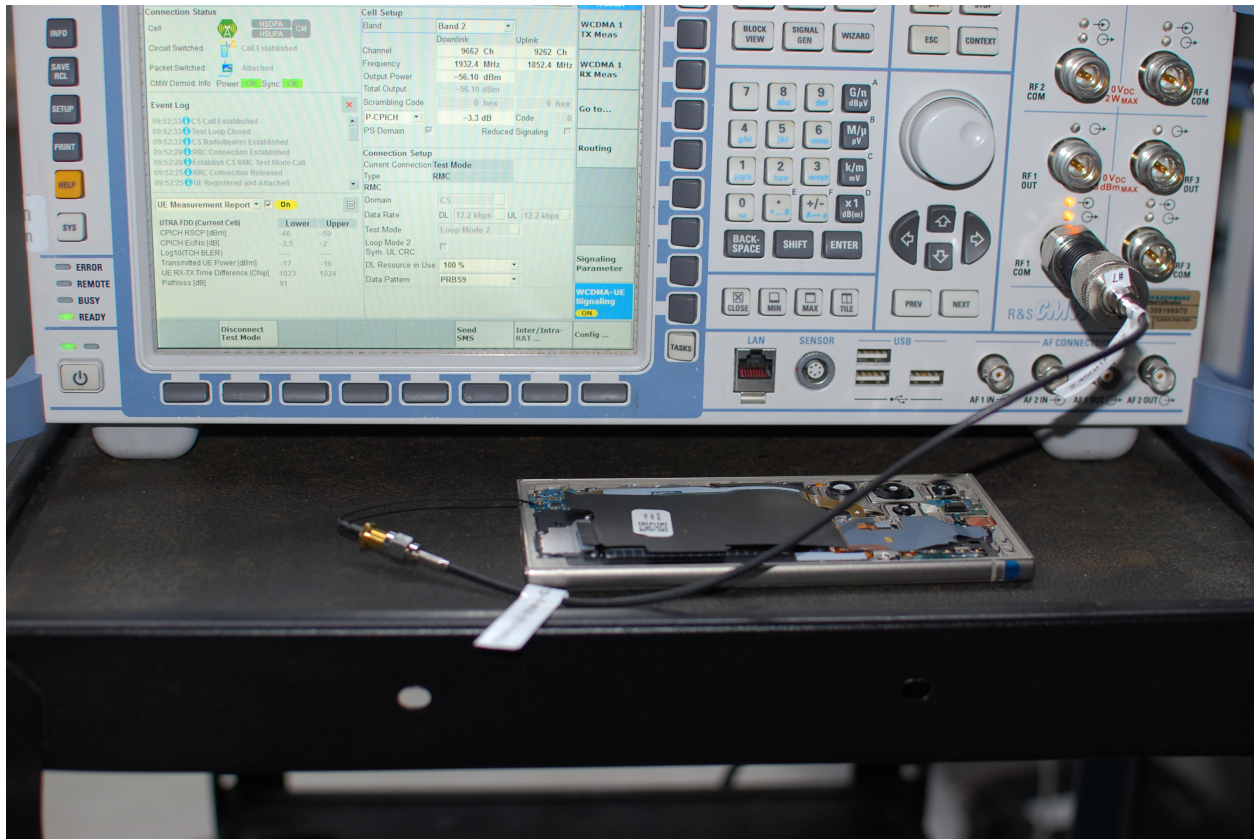
Figure 12-1 Test Setup for peak power level requirements
