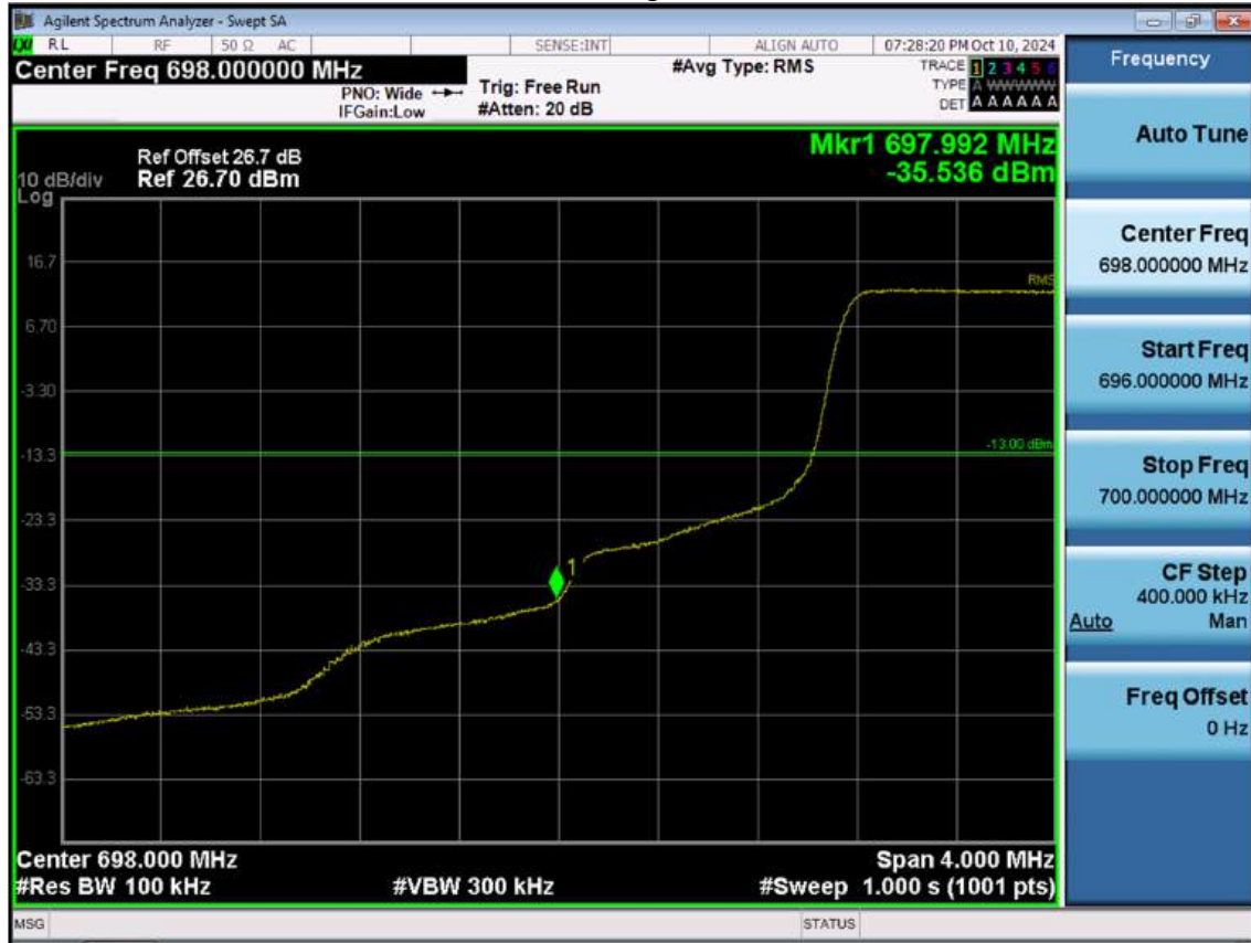
LTE B12_1.4M_Band Edge_Low_QPSK_FullRB
