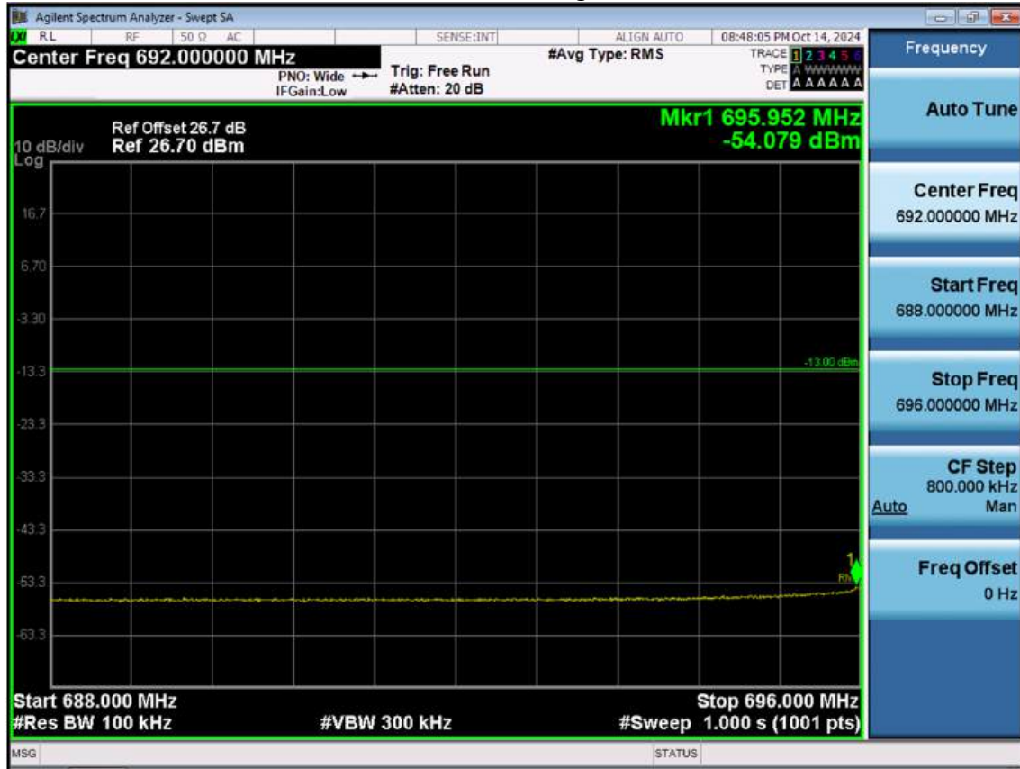
LTE B12_1.4M_Extended Band Edge_Low_QPSK_FullRB
