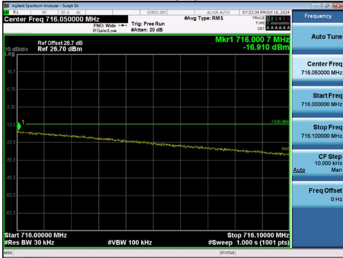
LTE B12_1.4M_Band Edge_High_QPSK_1RB(1)
