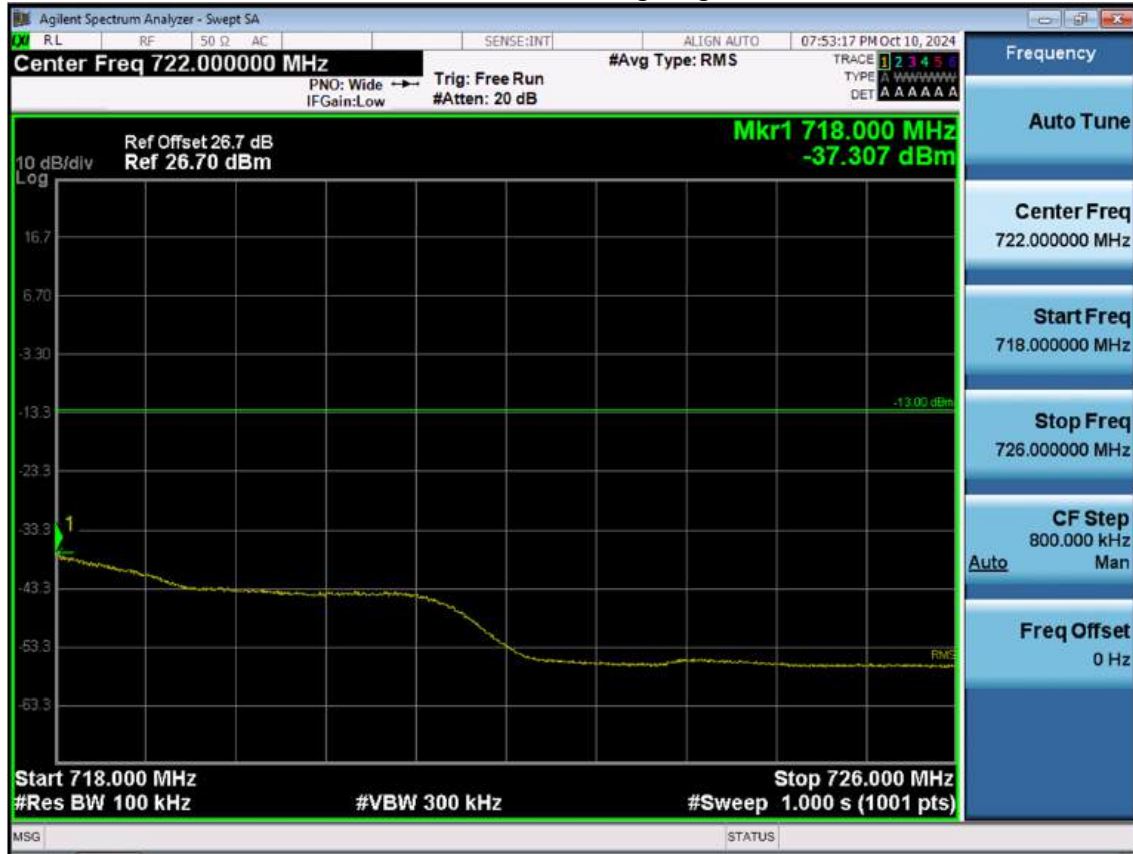
LTE B12_10 M_Extended Band Edge_High_QPSK_FullRB
