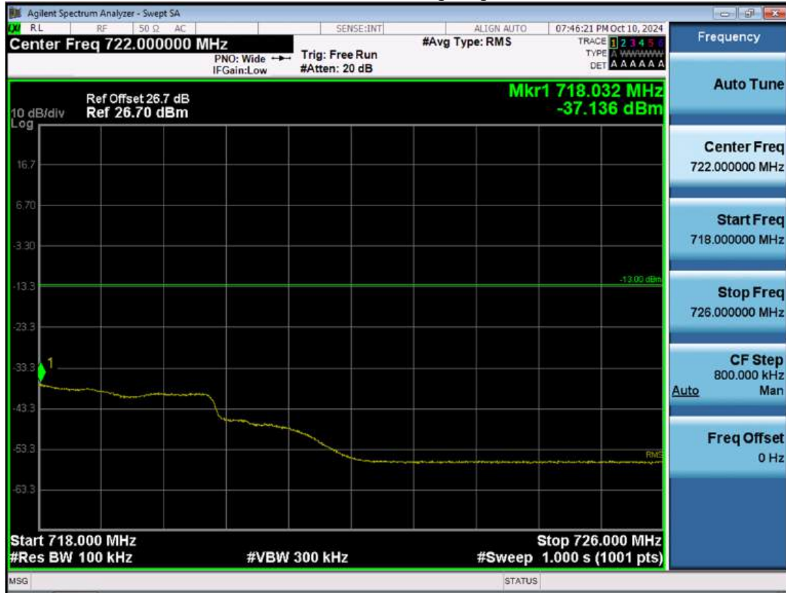
LTE B12_5 M_Extended Band Edge_High_QPSK_FullRB
