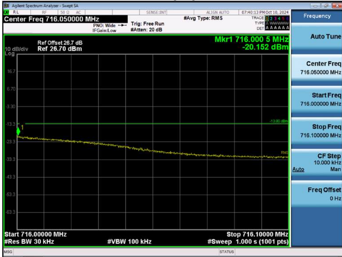
LTE B12_3 M_Band Edge_High_QPSK_1RB(1)
