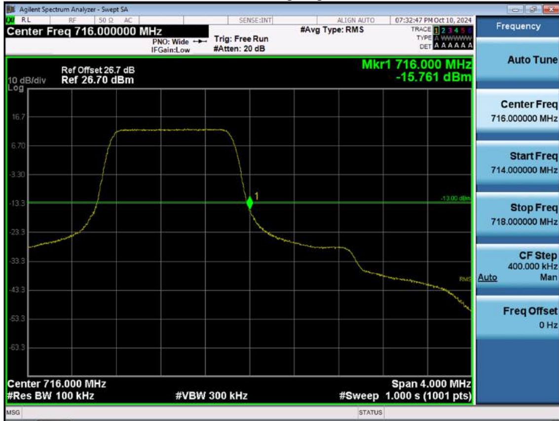
LTE B12_1.4M_Band Edge_High_QPSK_FullRB
