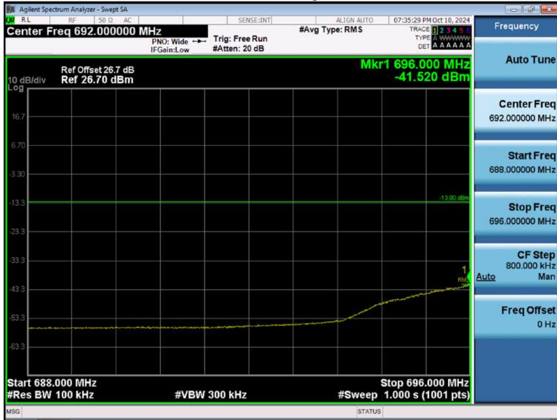
LTE B12_3 M_Extended Band Edge_Low_QPSK_FullRB
