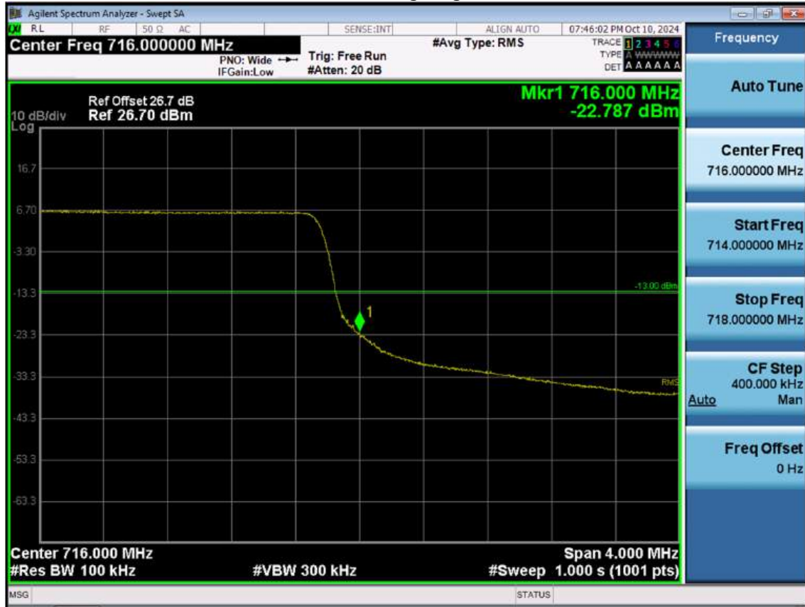
LTE B12_5 M_Band Edge_High_QPSK_FullRB
