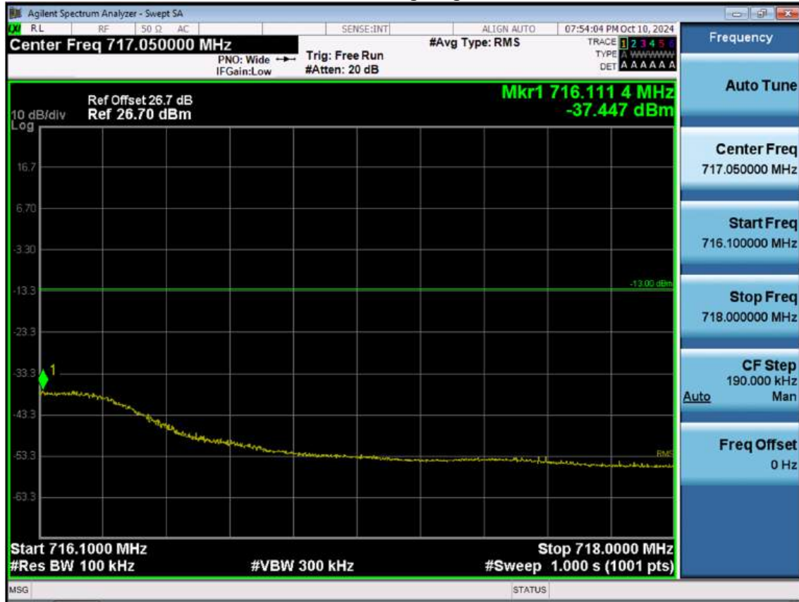
LTE B12_10 M_Band Edge_High_QPSK_1RB(2)
