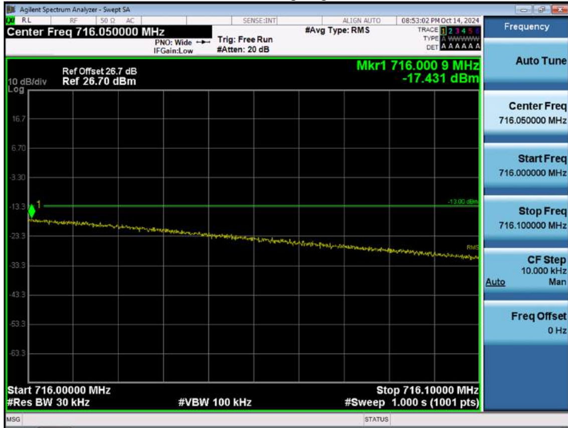
LTE B12_1.4M_Band Edge_High_QPSK_1RB(1)
