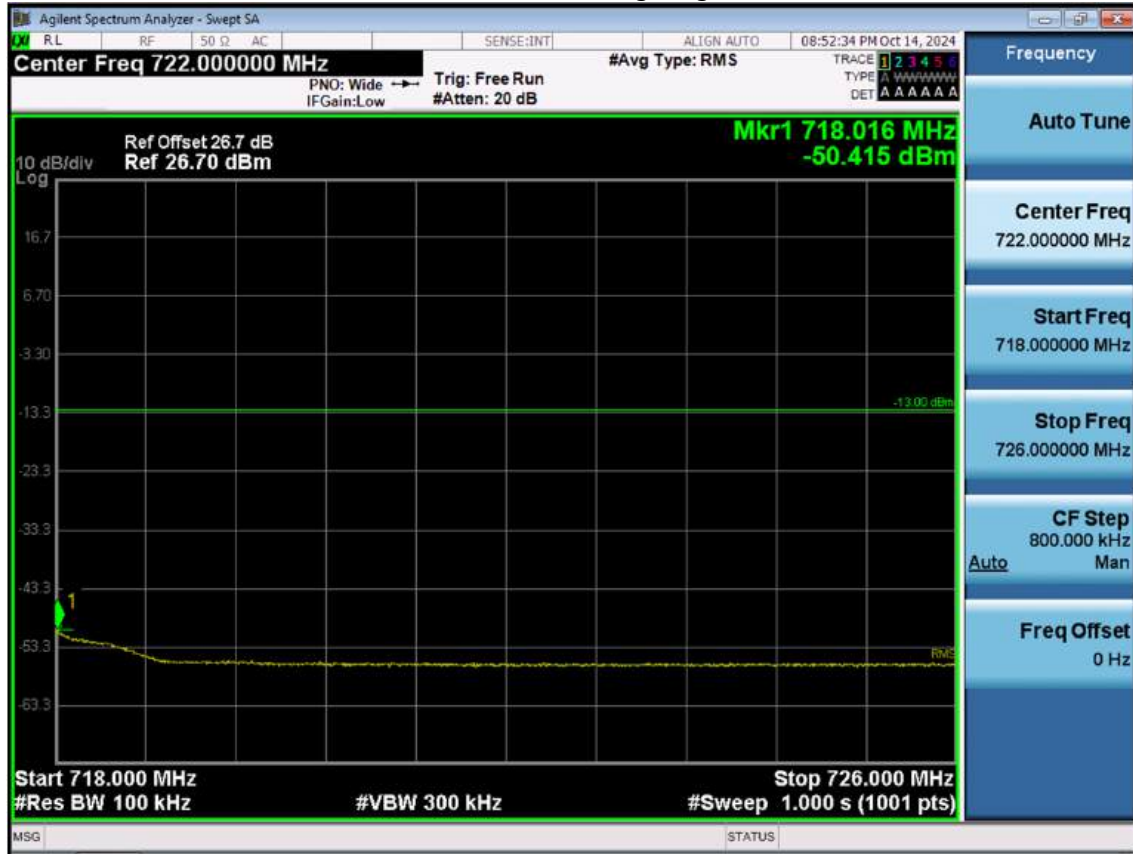
LTE B12_1.4M_Extended Band Edge_High_QPSK_FullRB
