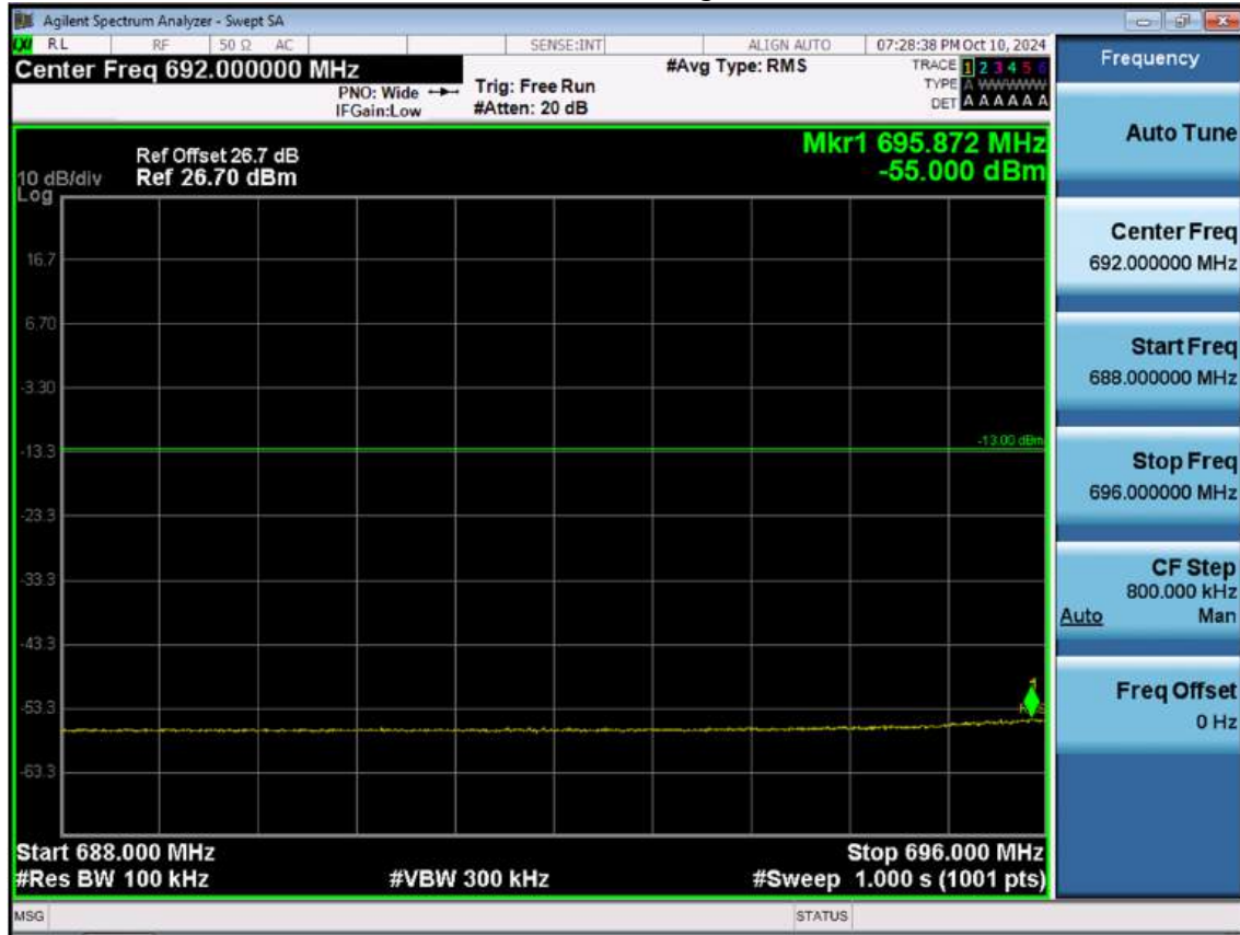
LTE B12_1.4M_Extended Band Edge_Low_QPSK_FullRB
