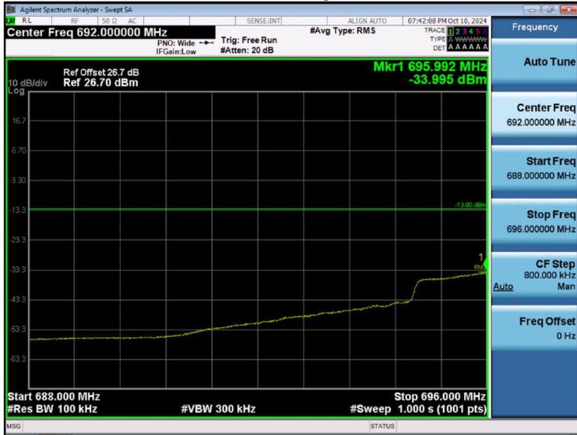
LTE B12_5 M_Extended Band Edge_Low_QPSK_FullRB
