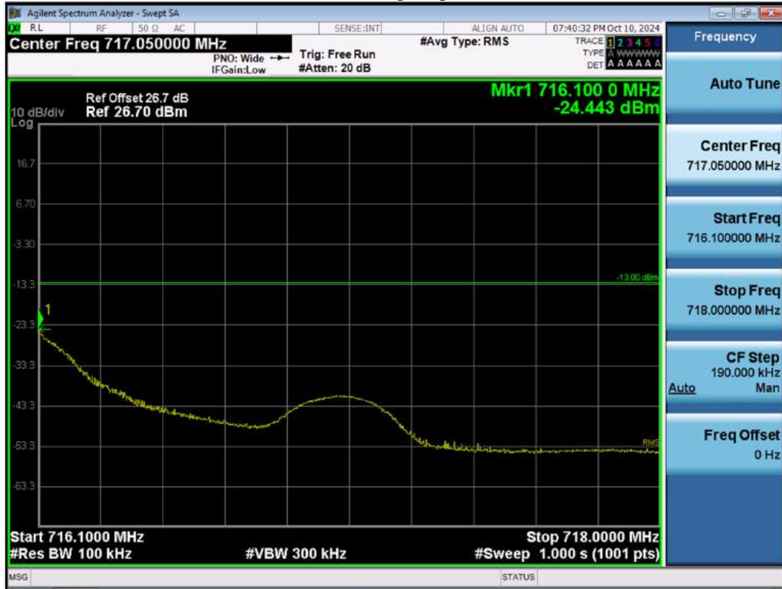
LTE B12_3 M_Band Edge_High_QPSK_1RB(2)
