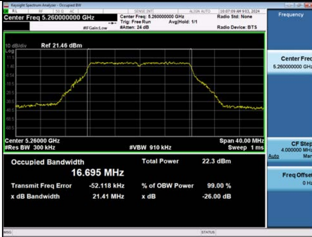
802.11ac(VHT20) 26 dB Bandwidth (CH 169)
