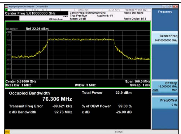
802.11ac(VHT80) 26 dB Bandwidth (CH 122)
