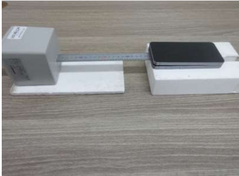
Edge 1 + TA : 20 cm (The distance between the DUT and the probe is 20 cm.)
