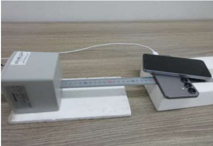
Edge 2 + TA : 20 cm (The distance between the DUT and the probe is 20 cm.)
