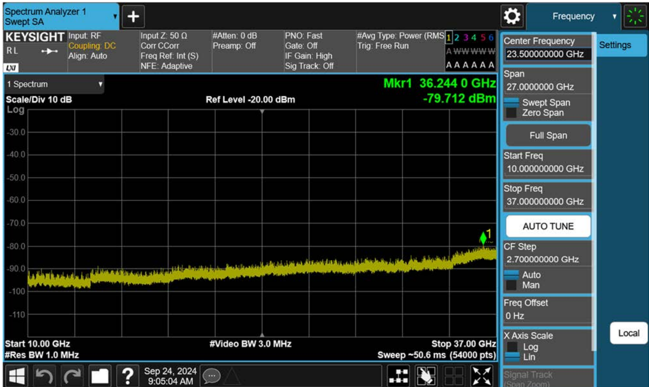
BAND 48. Conducted Spurious Plot 2 (5 MHz Ch. 55990 QPSK RB 1, Offset 0)
