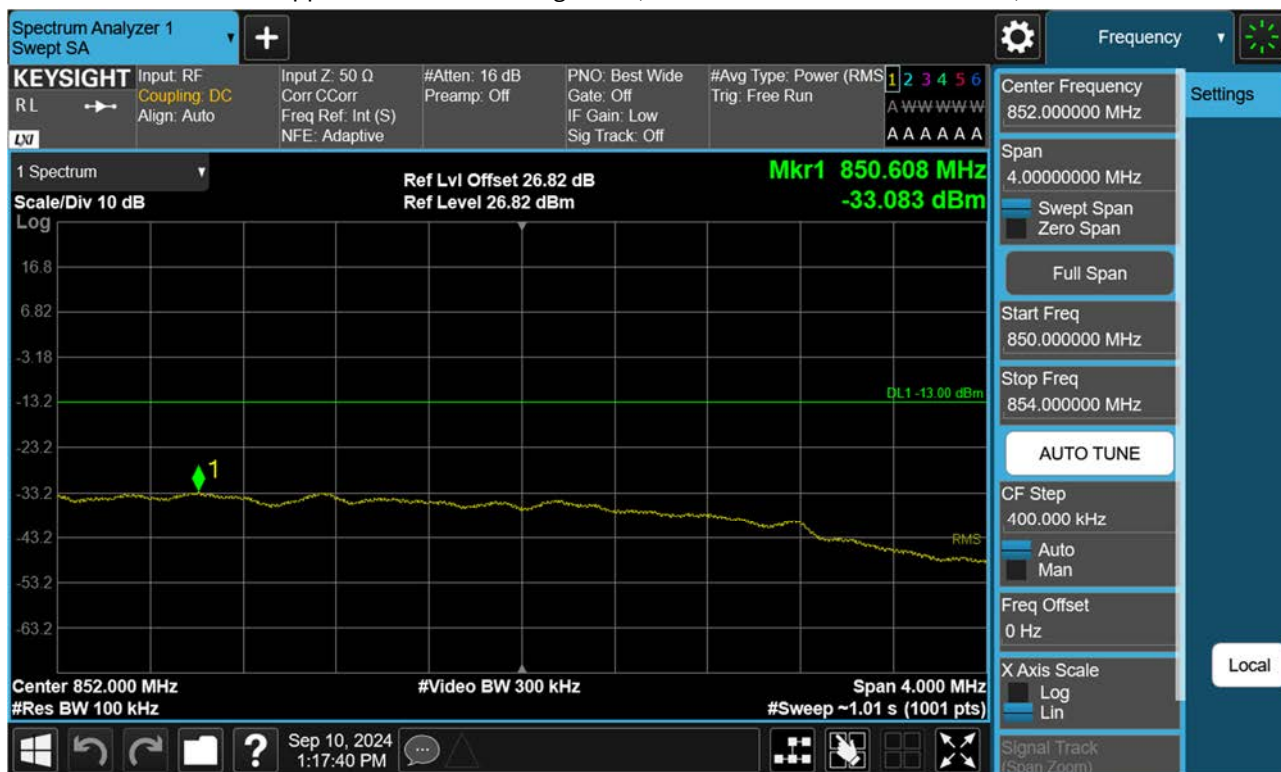
Upper Extended Band Edge Plot (5 M BW Ch.169300 BPSK_RB 25_0)
