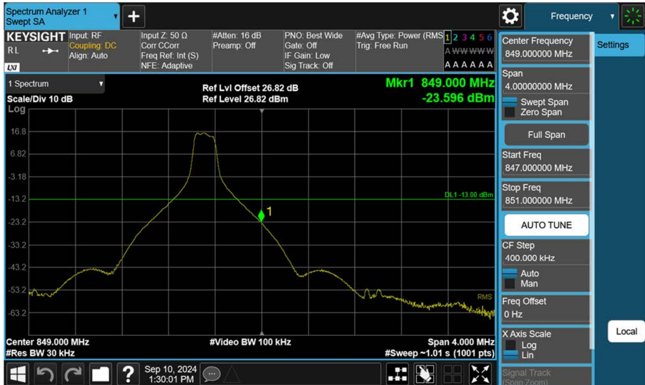
Upper Band Edge Plot (15 M BW Ch.168300 BPSK_RB 1_Offset 74)
