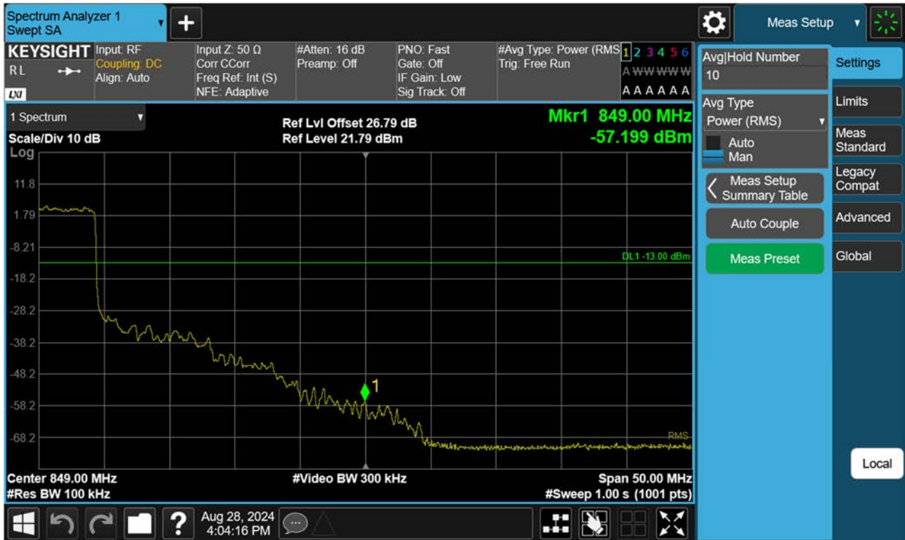
Sub6 n26. Upper Band Edge Plot (10 M BW Ch.164800 BPSK_RB50_Offset 0)
