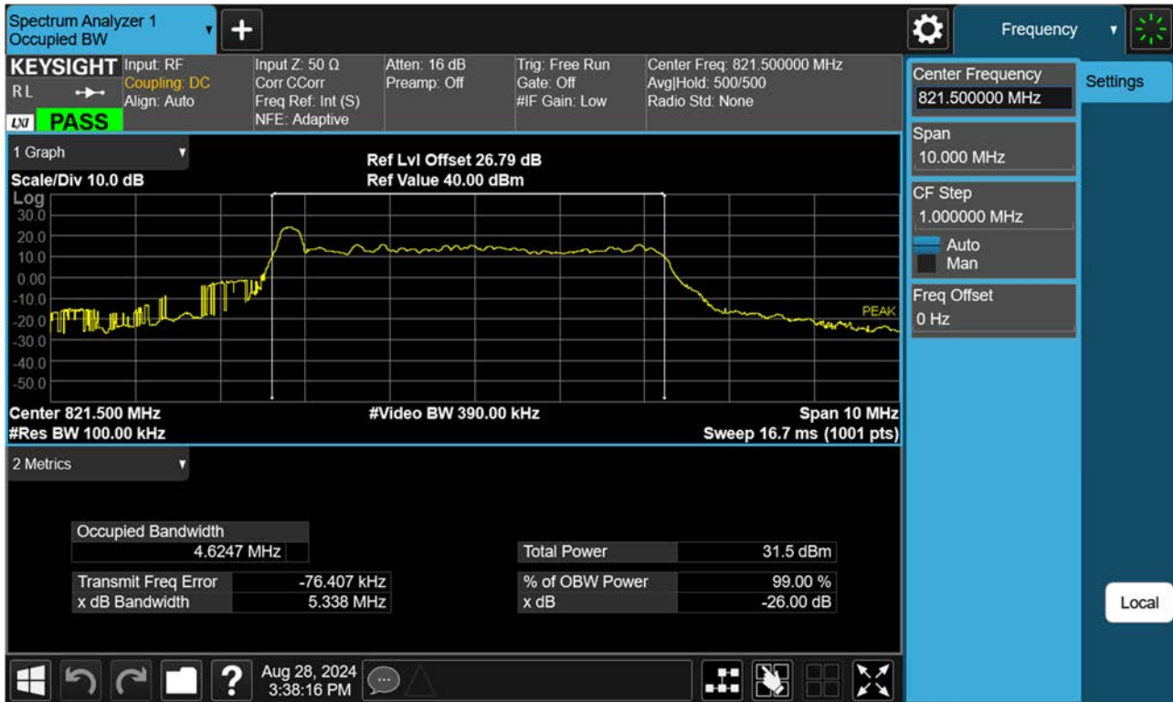
Sub6 n26. Occupied Bandwidth Plot (5 M BW Ch.164300 16QAM RB 25_0)
