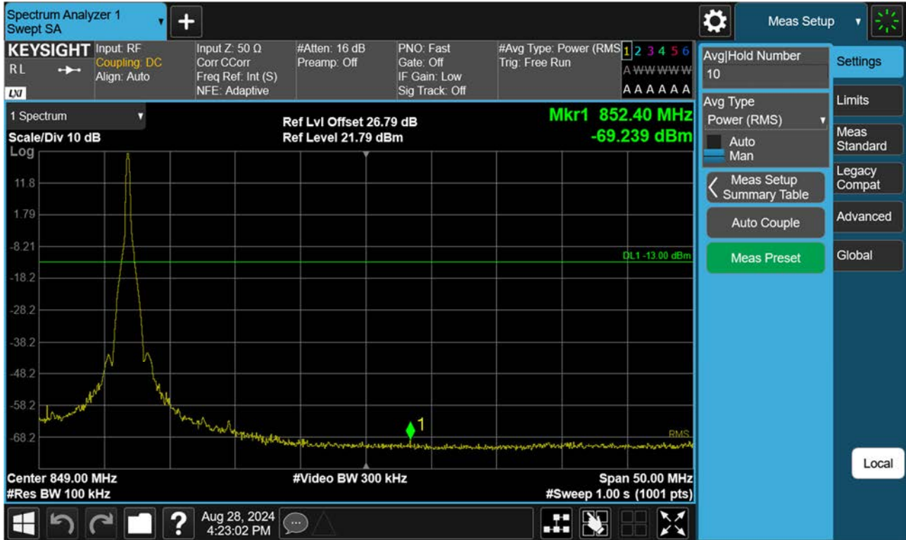
Sub6 n26. Upper Band Edge Plot (15 M BW Ch.164800 BPSK_RB1_Offset 78)
