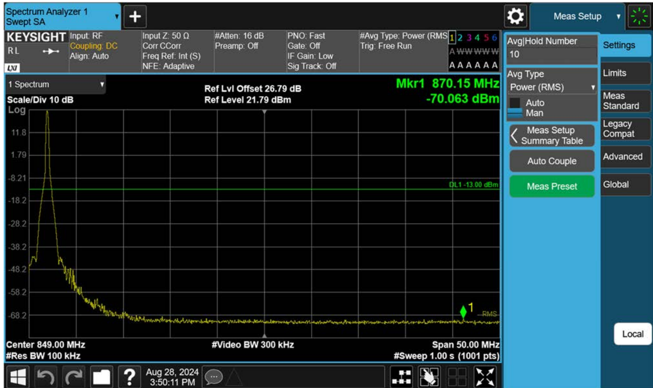
Sub6 n26. Upper Band Edge Plot (5 M BW Ch.164800 BPSK_RB1_Offset 24)
