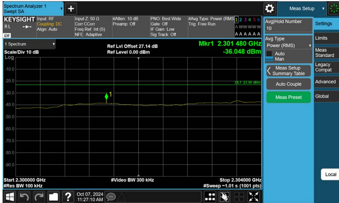
NR30_5 M_Band Edge(2300MHz-2304MHz)_Low_BPSK_FullRB
