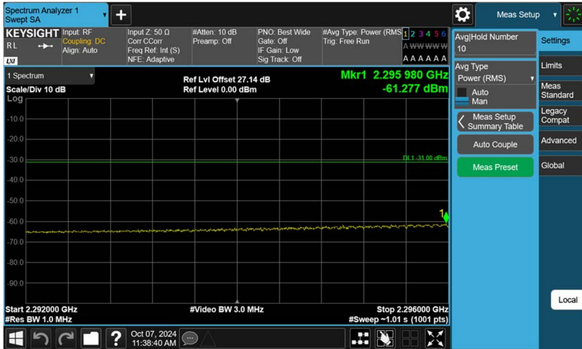
NR30_5 M_Band Edge(2292MHz-2296MHz)_Mid_BPSK_1RB
