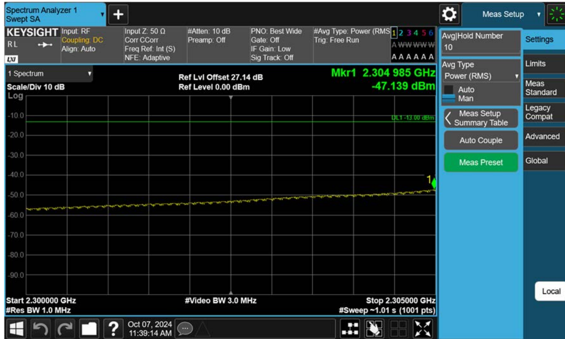
NR30_5 M_Band Edge(2300MHz-2305MHz)_Mid_BPSK_1RB
