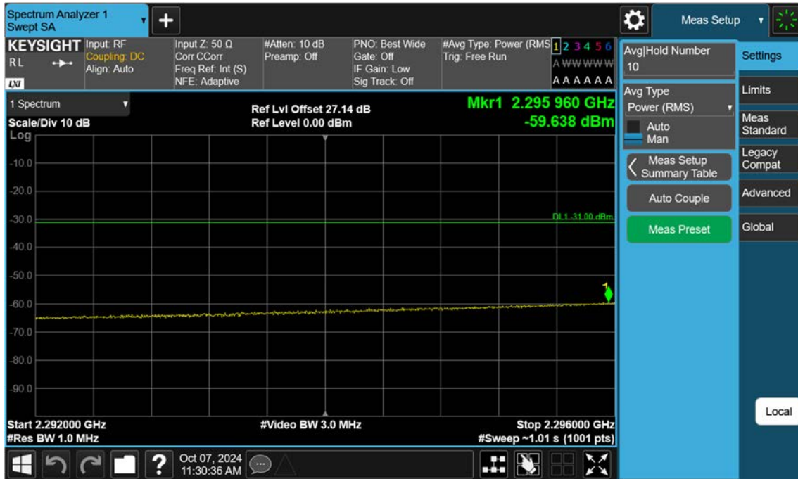
NR30_5 M_Band Edge(2292MHz-2296MHz)_Low_BPSK_1RB
