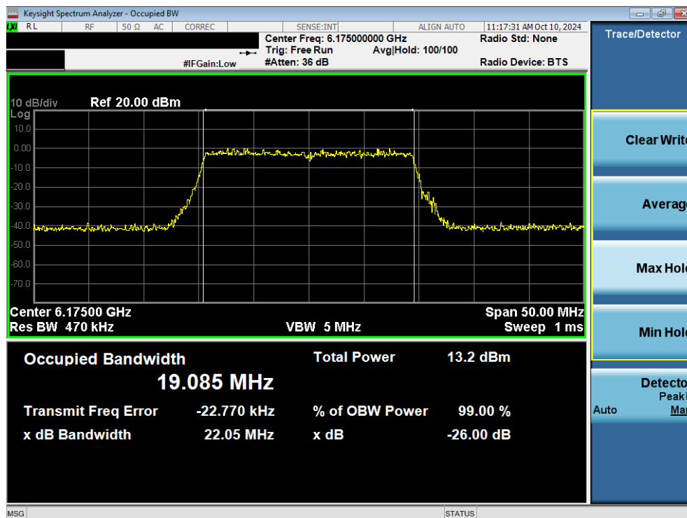
Plot 7-18. 26dB Bandwidth Plot MIMO ANT2 (20MHz 802.11ax/be (UNII Band 5) – Ch. 45) - VLP
