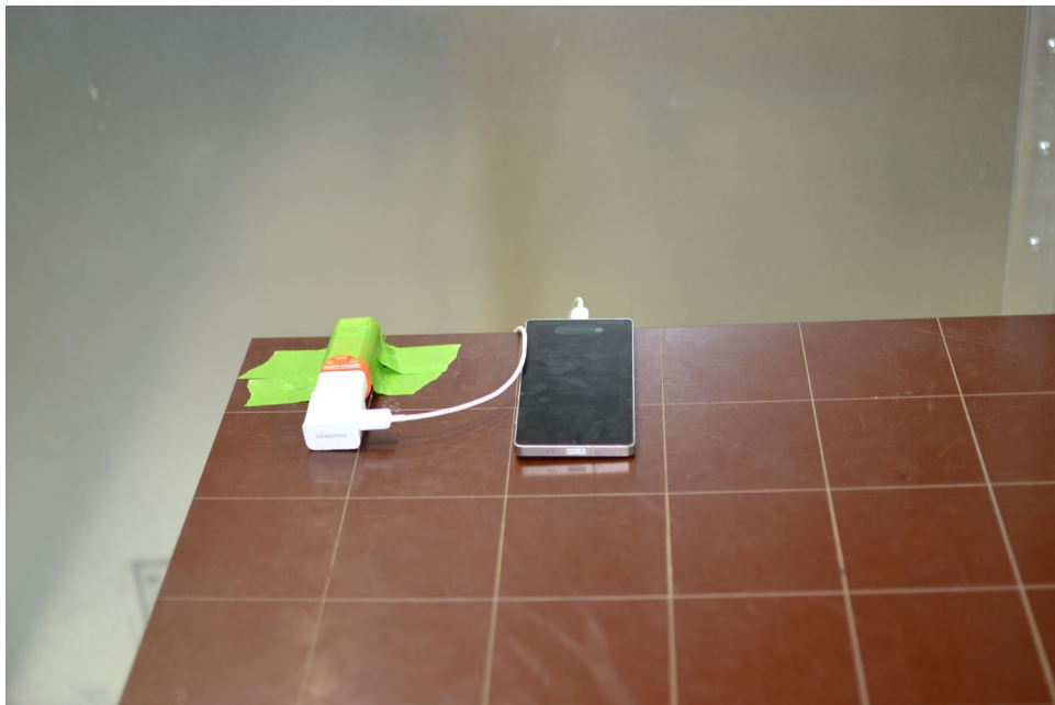
Figure 2. Test Setup – ACLC– <30MHz
