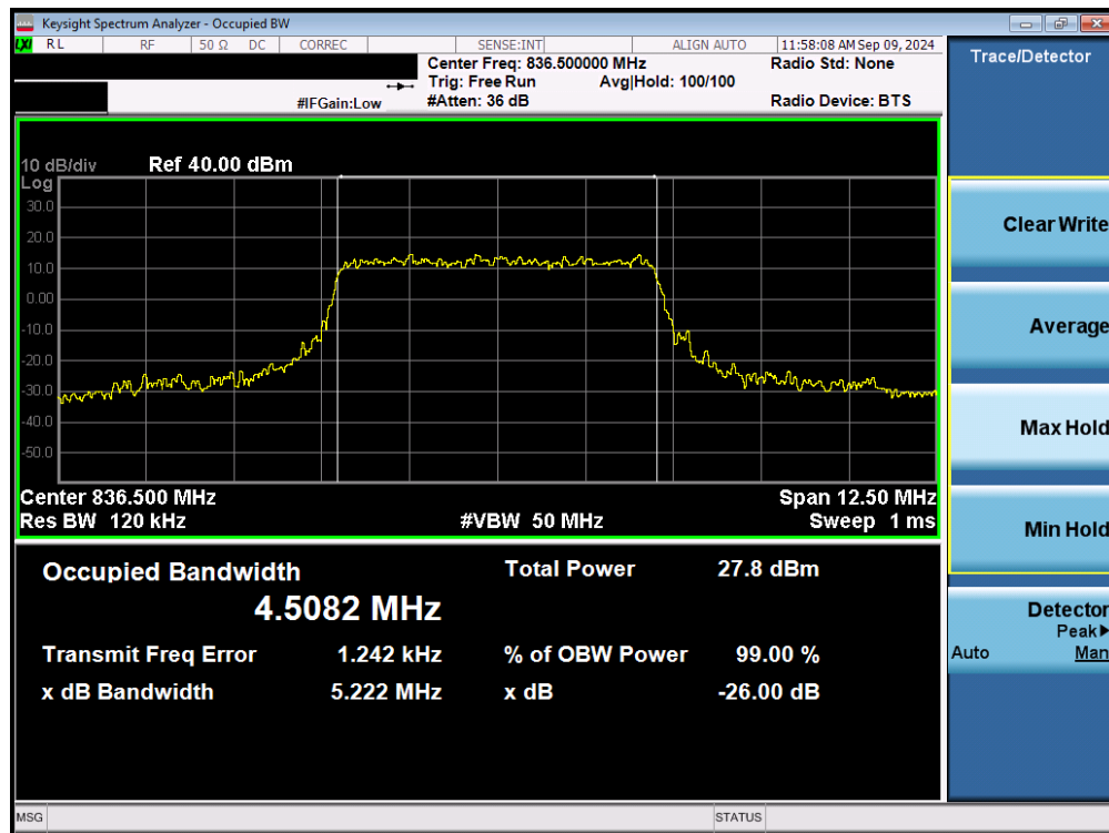
Plot 7-49. Occupied Bandwidth Plot (NR Band n26/5 - 5MHz QPSK - Full RB - Ant2)
