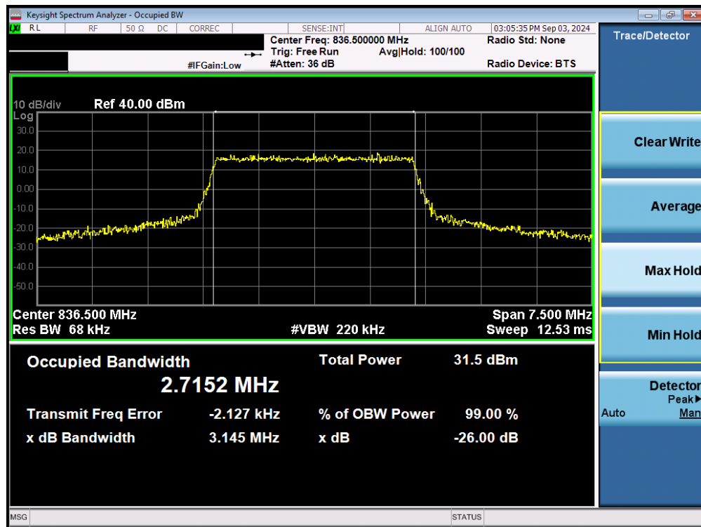
Plot 7-10. Occupied Bandwidth Plot (LTE Band 26/5 - 3MHz QPSK - Full RB - Ant1)
