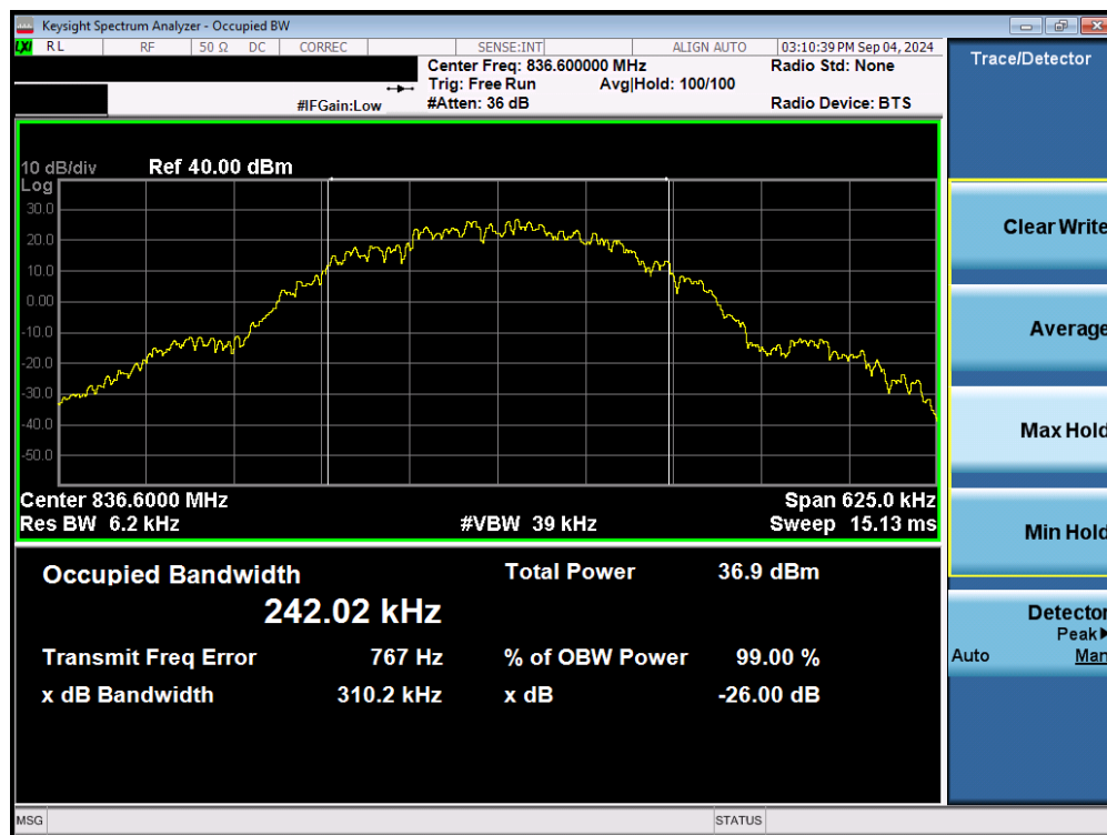
Plot 7-1. Occupied Bandwidth Plot (GPRS, Ch. 190 – Ant1)
