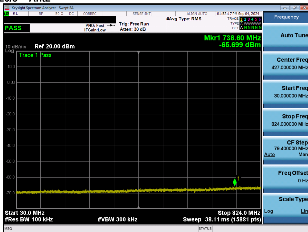
Plot 7-69. Conducted Spurious Plot (LTE Band 26/5 - 10MHz QPSK - 1 RB - Mid Channel – Ant2)
