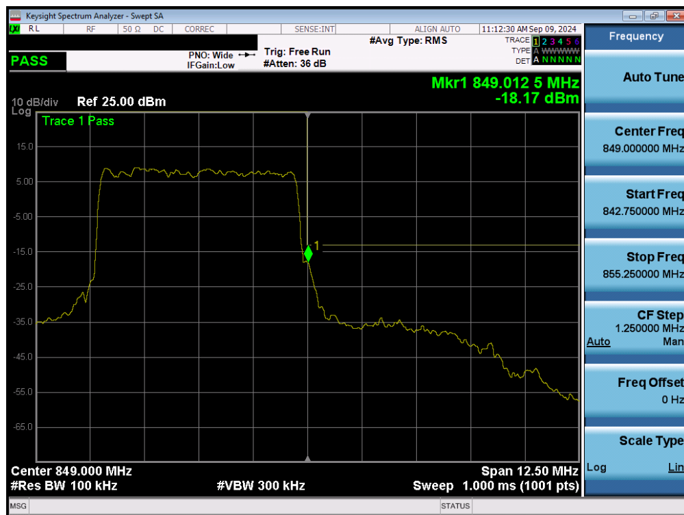
Plot 7-82. Upper Band Edge Plot (NR Band n26/5 – 5.0MHz - Full RB - Ant1)
