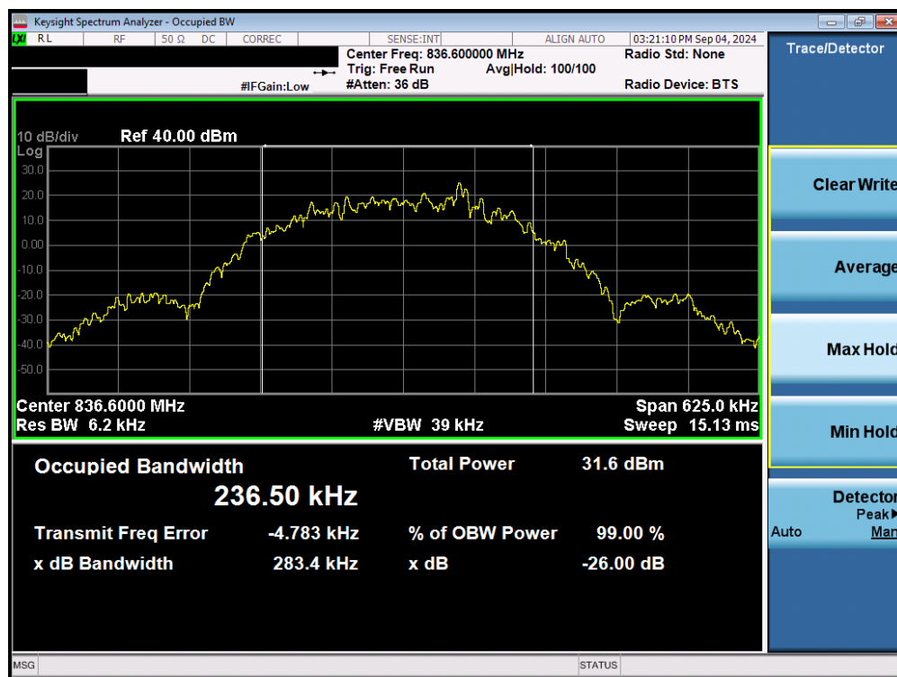
Plot 7-2. Occupied Bandwidth Plot (EDGE, Ch. 190 – Ant1)
