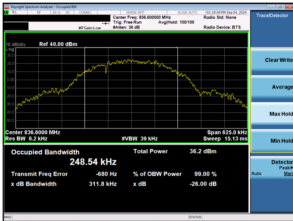
Plot 7-26. Occupied Bandwidth Plot (GPRS, Ch. 190 – Ant2)
