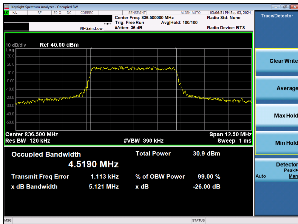
Plot 7-8. Occupied Bandwidth Plot (LTE Band 26/5 - 5MHz QPSK - Full RB - Ant1)
