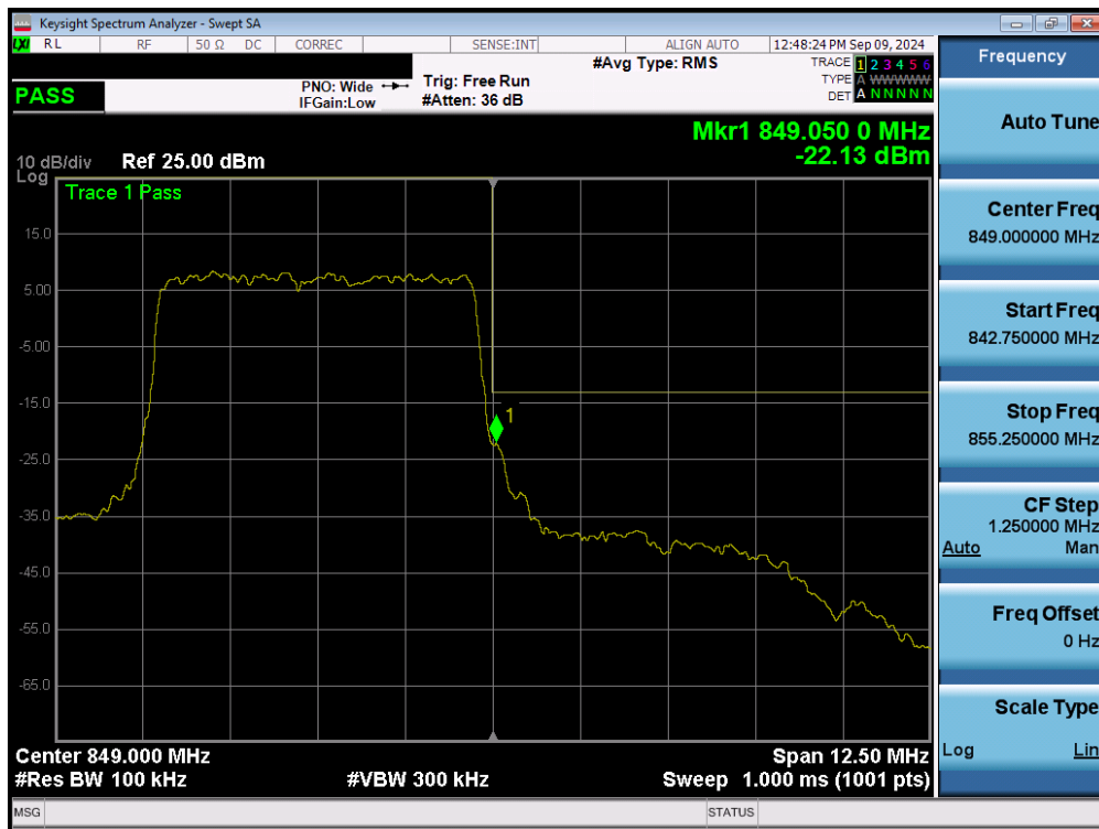
Plot 7-90. Upper Band Edge Plot (NR Band n26/5 – 5.0MHz - Full RB - Ant2)
