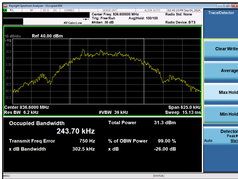
Plot 7-27. Occupied Bandwidth Plot (EDGE, Ch. 190 – Ant2)
