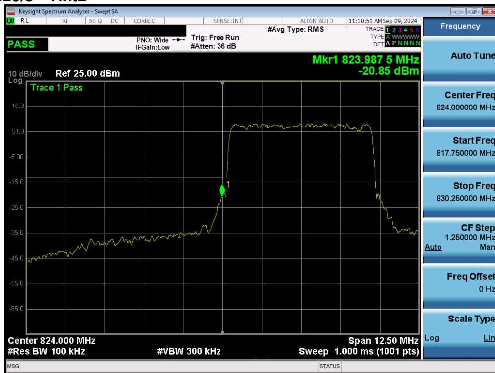
Plot 7-81. Lower Band Edge Plot (NR Band n26/5 – 5.0MHz - Full RB - Ant1)
