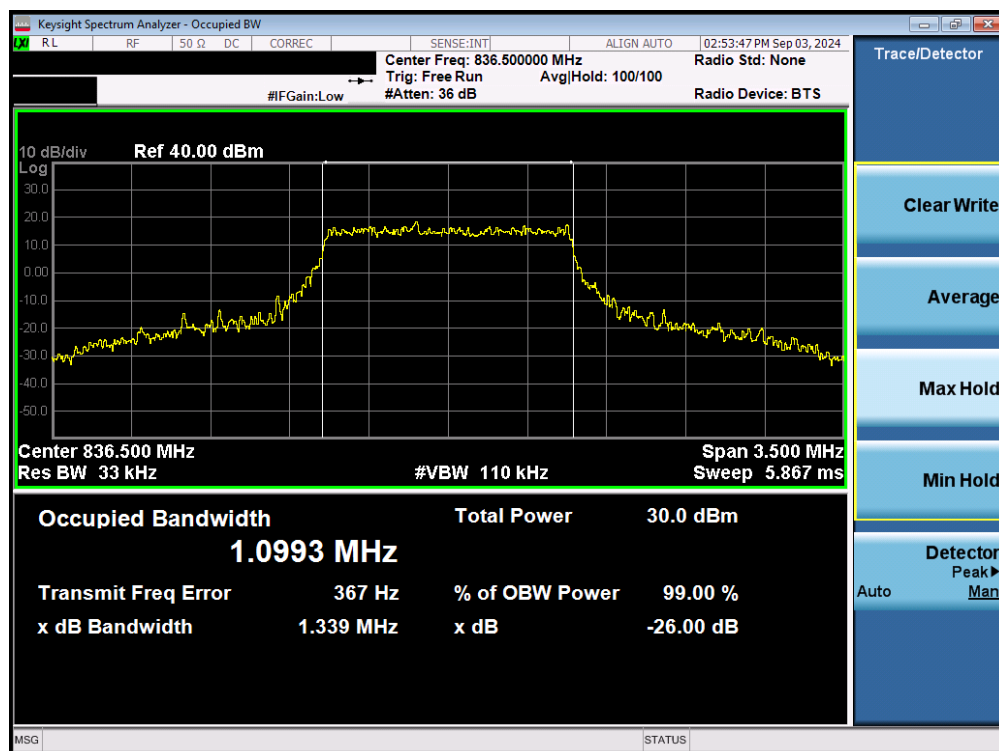
Plot 7-13. Occupied Bandwidth Plot (LTE Band 26/5 - 1.4MHz 16-QAM - Full RB - Ant1)
