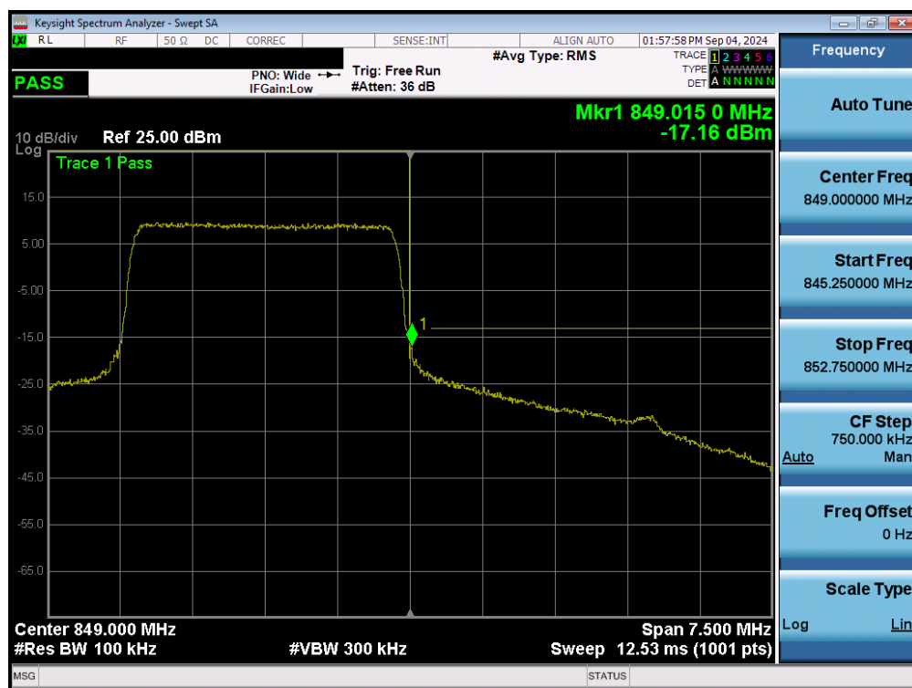
Plot 7-88. Upper Band Edge Plot (LTE Band 26/5 - 3MHz QPSK – Full RB - Ant2)
