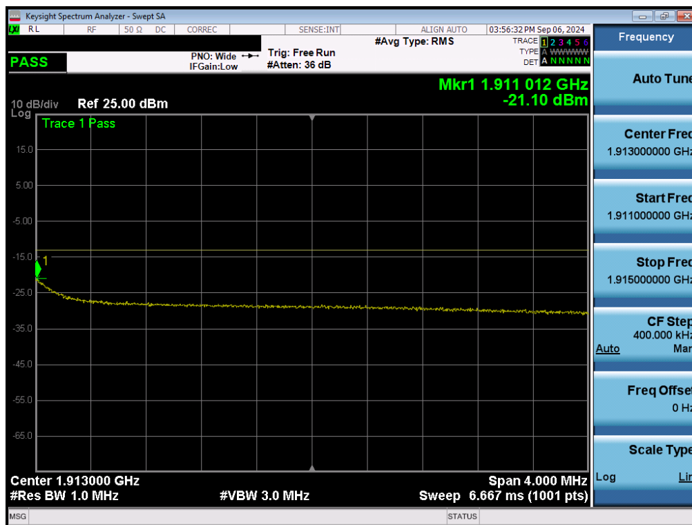
Plot 7-157. Extended Upper Band Edge Plot (NR Band n2 - 10MHz QPSK – Full RB - Ant2)
