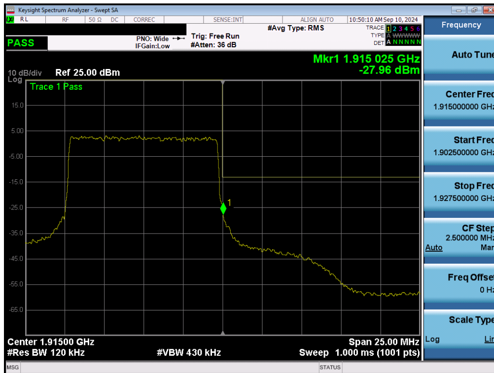
Plot 7-152. Upper Band Edge Plot (NR Band n25 - 10MHz QPSK – Full RB - Ant1)
