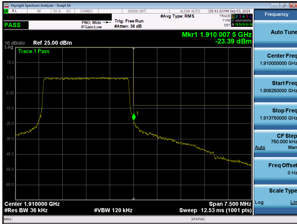
Plot 7-144. Upper Band Edge Plot (LTE Band 2 - 3MHz QPSK – Full RB - Ant2)
