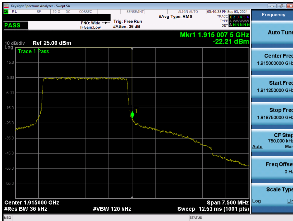
Plot 7-146. Upper Band Edge Plot (LTE Band 25 - 3MHz QPSK – Full RB - Ant2)
