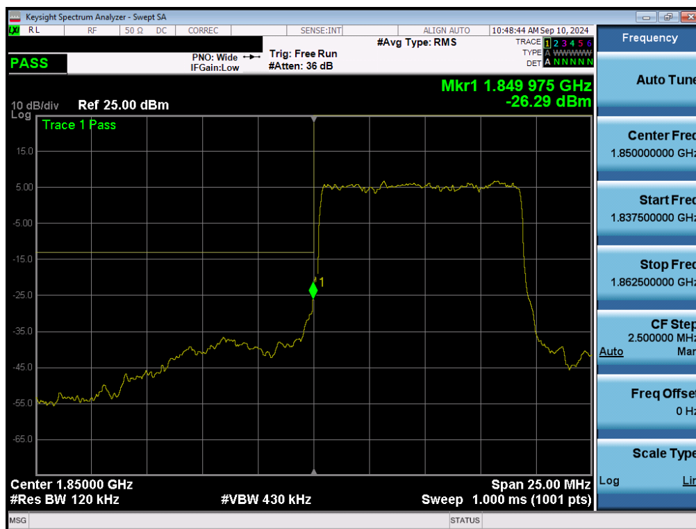
Plot 7-148. Lower Band Edge Plot (NR Band n25/2 - 10MHz QPSK – Full RB - Ant1)
