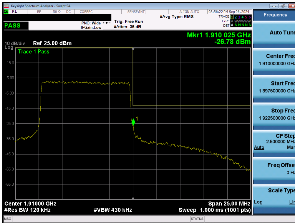
Plot 7-156. Upper Band Edge Plot (NR Band n2 - 10MHz QPSK – Full RB - Ant2)
