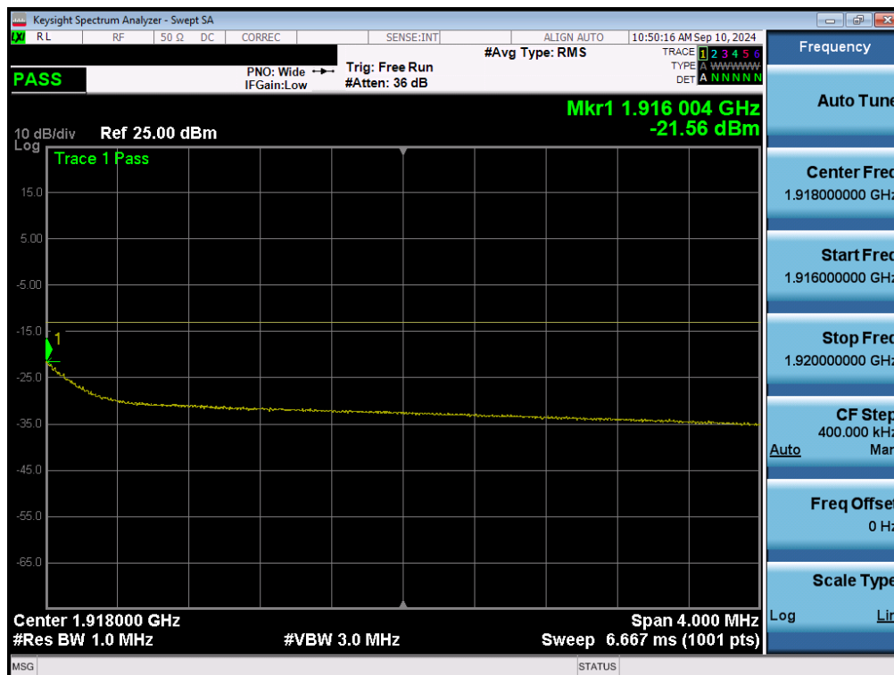
Plot 7-153. Extended Upper Band Edge Plot (NR Band n25 - 10MHz QPSK – Full RB - Ant1)
