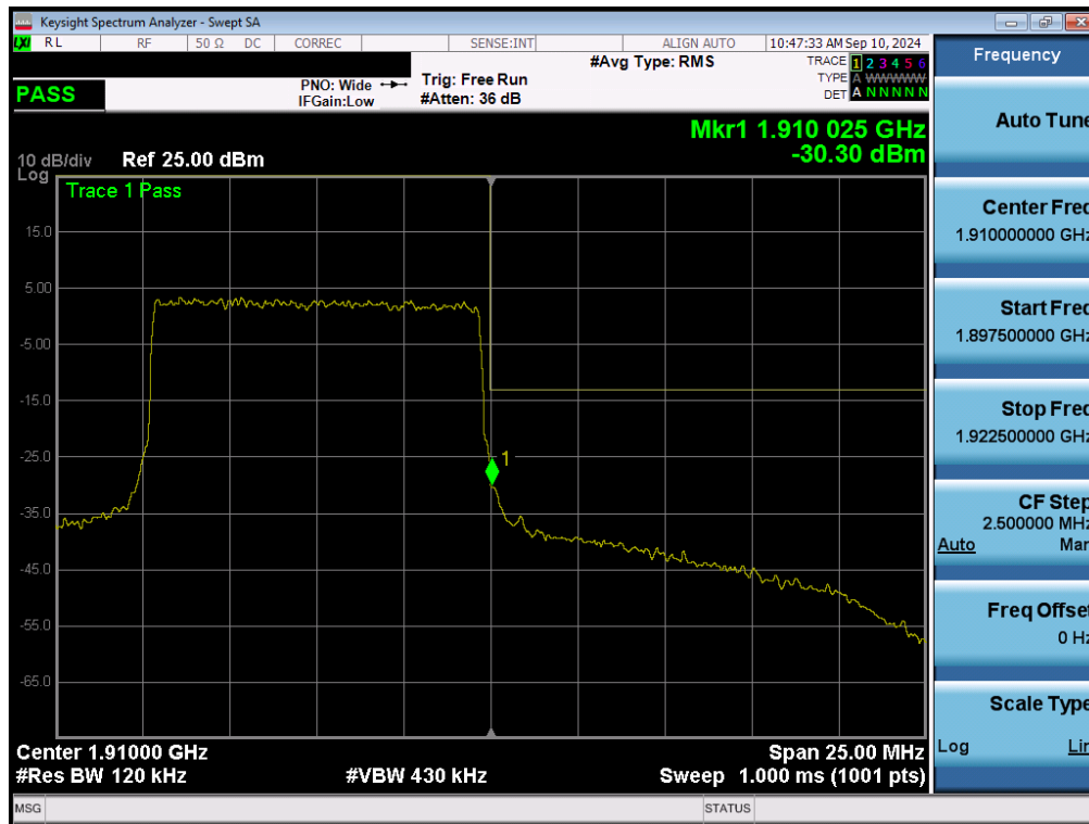
Plot 7-150. Upper Band Edge Plot (NR Band n2 - 10MHz QPSK – Full RB - Ant1)
