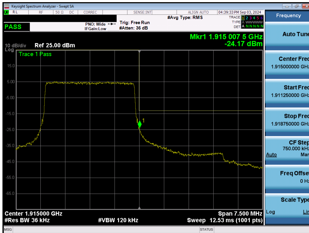
Plot 7-140. Upper Band Edge Plot (LTE Band 25 - 3MHz QPSK – Full RB - Ant1)
