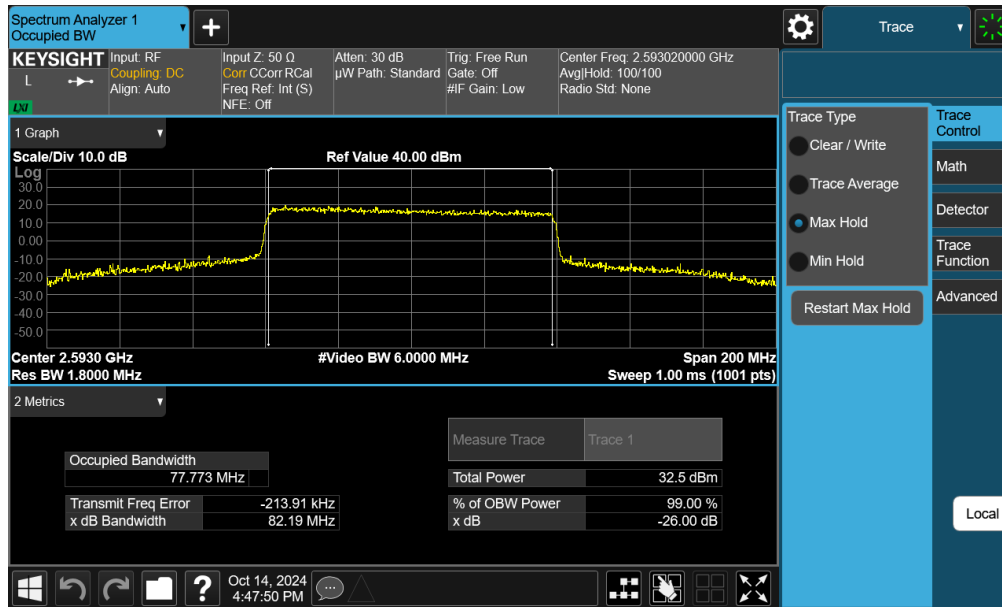
Plot 7-80. Occupied Bandwidth Plot (NR Band n41 - 80MHz 16-QAM - Full RB - Ant F)
