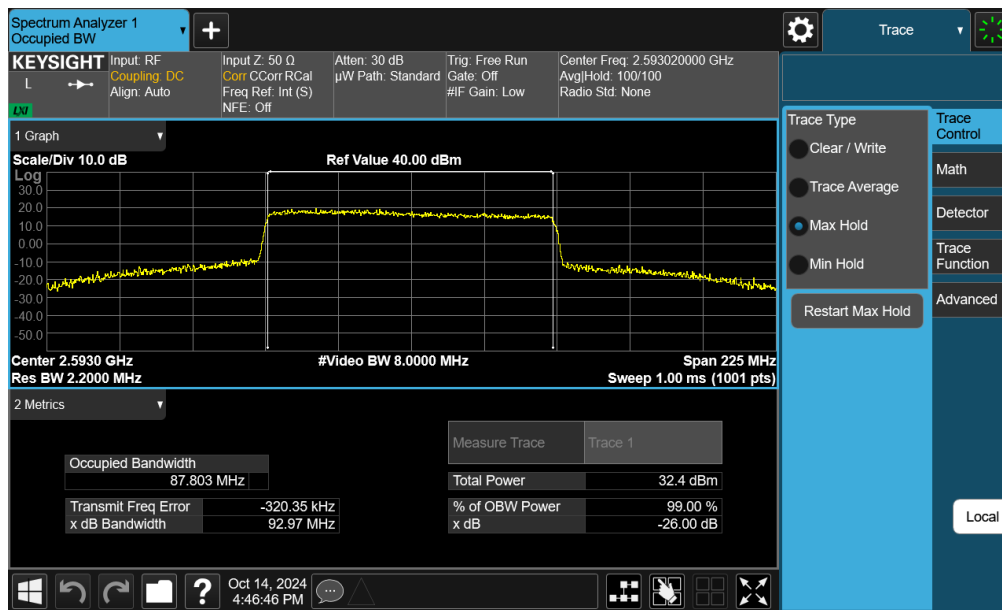
Plot 7-77. Occupied Bandwidth Plot (NR Band n41 - 90MHz 16-QAM - Full RB - Ant F)
