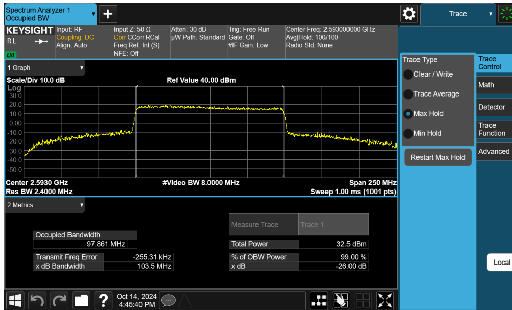
Plot 7-74. Occupied Bandwidth Plot (NR Band n41 - 100MHz 16-QAM - Full RB - Ant F)
