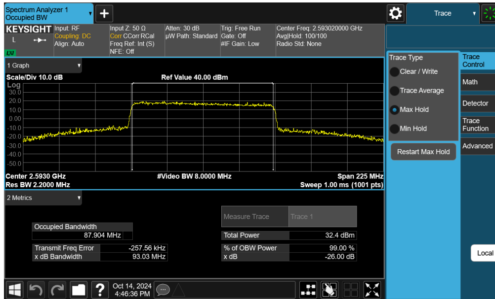
Plot 7-76. Occupied Bandwidth Plot (NR Band n41 - 90MHz QPSK - Full RB - Ant F)
