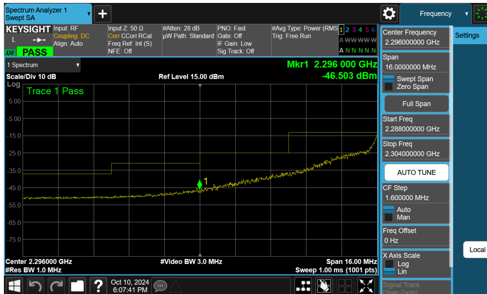
Plot 7-290. Extended Lower Band Edge Plot (NR Band n30 - 5MHz CP-OFDM-QPSK – Full RB - Ant F)
