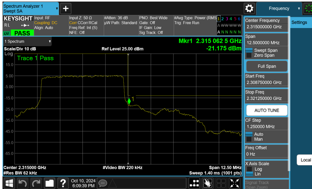
Plot 7-291. Upper Band Edge Plot (NR Band n30 - 5MHz DFT-s-OFDM-QPSK – Full RB - Ant F)
