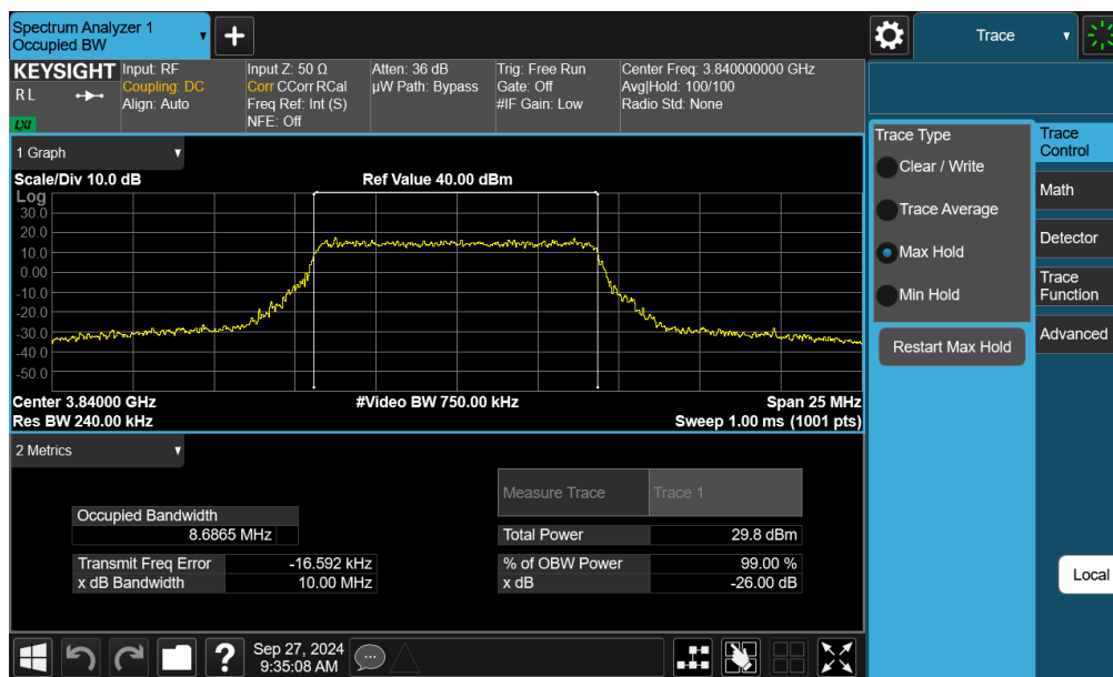
Plot 7-80. Occupied Bandwidth Plot (NR Band n77 C-band - 10MHz 16-QAM - Full RB - Ant F)
