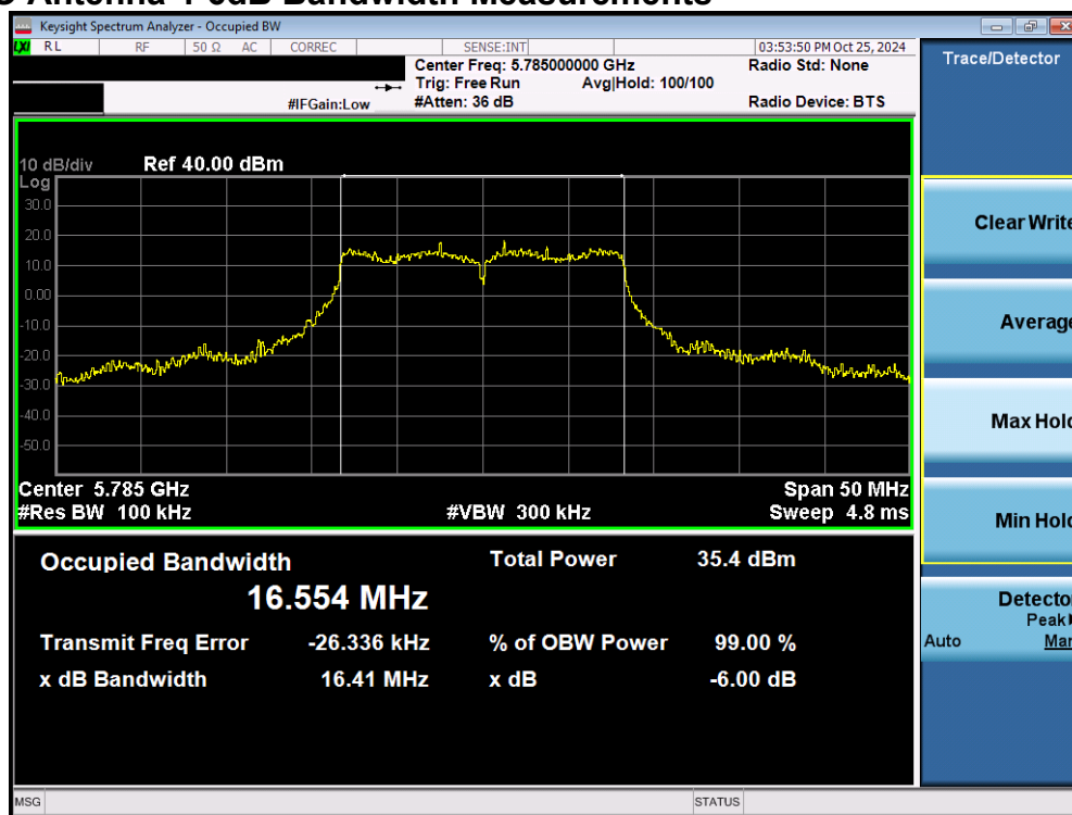
Plot 7-23. 6dB Bandwidth Plot MIMO ANT1 (20MHz 802.11a (UNII Band 3) – Ch.157)
