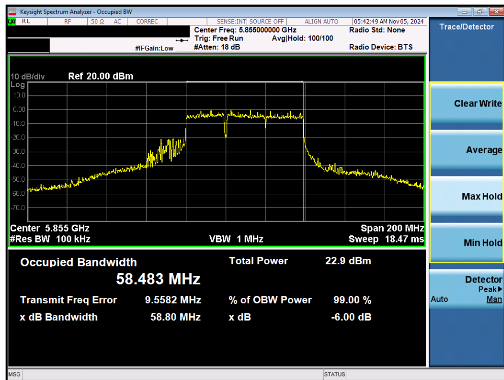
Plot 7-40. 6dB Bandwidth Plot MIMO ANT1 (80MHz 802.11be (20MHz Puncture) (UNII Band 3/4) – Ch. 171)
