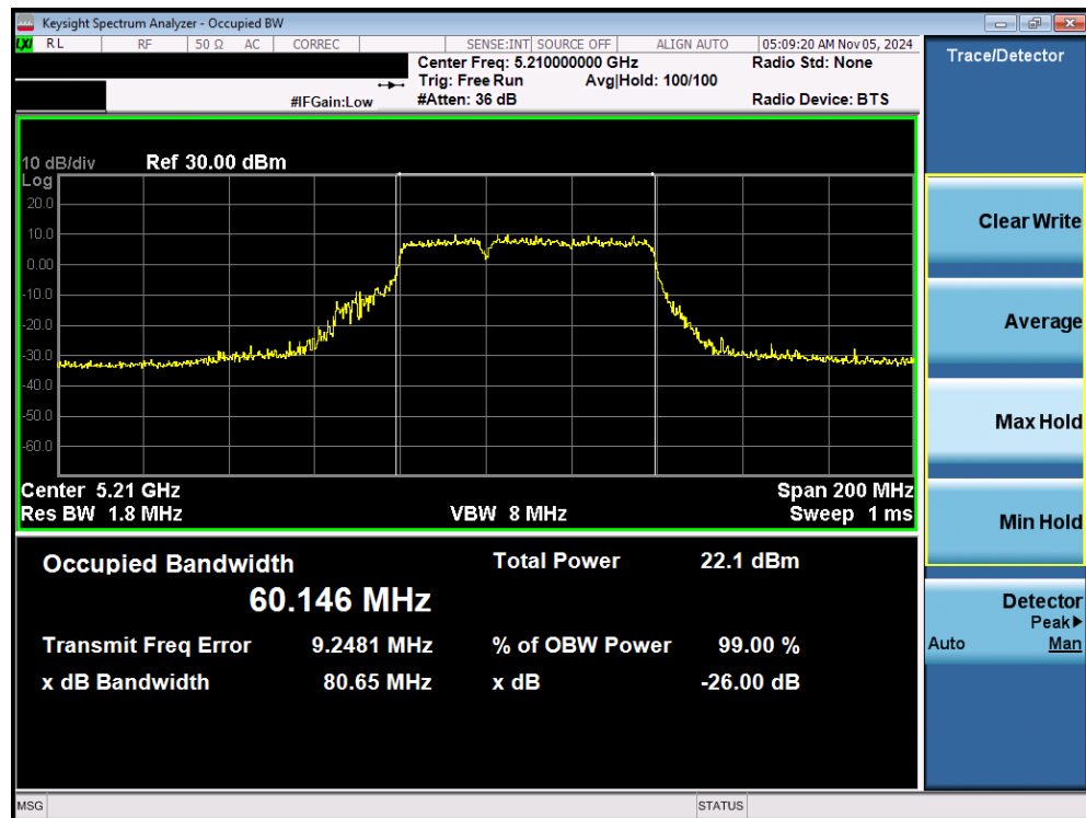
Plot 7-10. 26dB Bandwidth Plot MIMO ANT1 (80MHz 802.11be (20MHz Puncture) (UNII Band 1) – Ch. 42)
