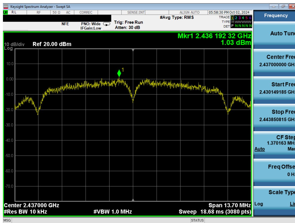
Plot 7-47. Power Spectral Density Plot (802.11b – Ch. 6) MIMO ANT2
