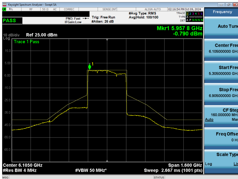
Plot 7-105. In Band Emissions Plot MIMO ANT2 (320MHz 802.11be (UNII Band 5) – Ch. 31) - SP
