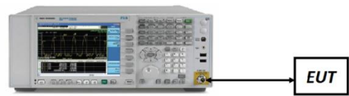
Figure 7-4. Test Instrument & Measurement Setup
