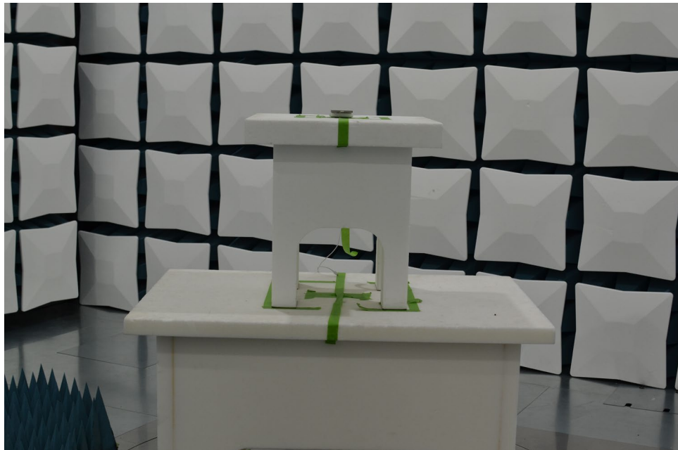
Figure 8. Test Setup – Wireless Charging Pad – 1GHz-40GHz
