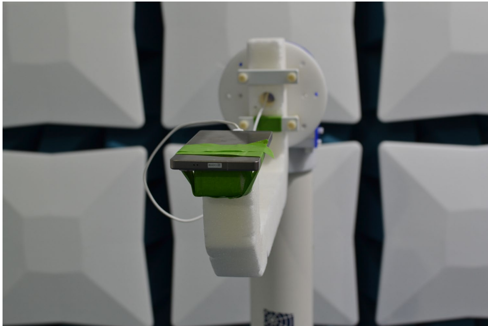
Figure 1. Test Setup – X Position – >18GHz
