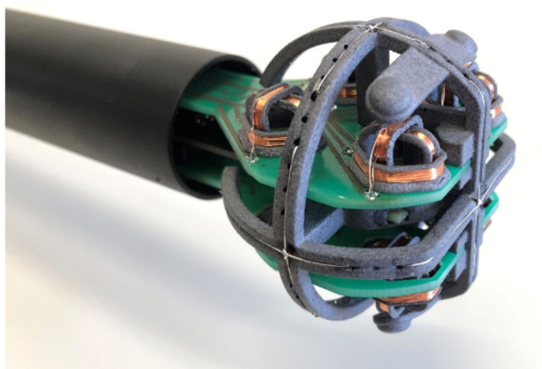
Figure 2-1 MAGPy-8H3D+E3 V2 Measurement Probe
